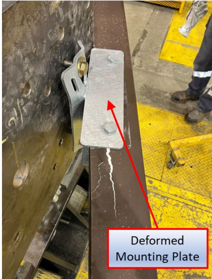
Figure E5. A representative post-test image showing typical deformation of the cross-arm mounting plate.
