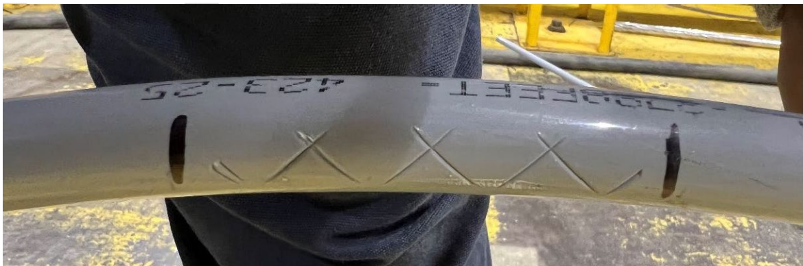
Figure 69. A representative post-test image showing superficial marks on the conductor at the Hendrix insulator grip location (17-kV 1/0 ACSR).
