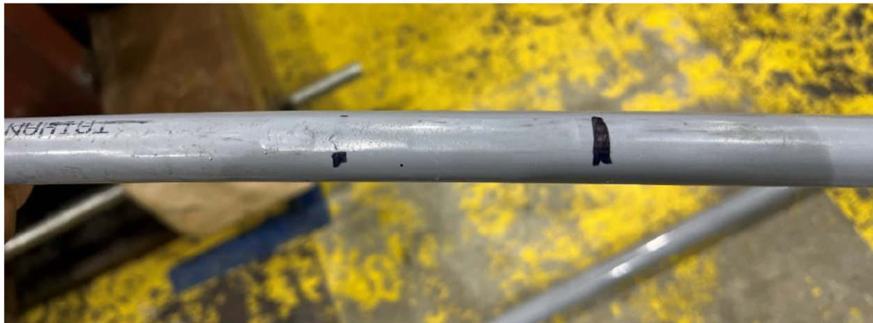
Figure 6-8: K-Line KL28SK - Typical 1/0 AWG ACSR (17 kV) Conductor Condition after Slip Test
