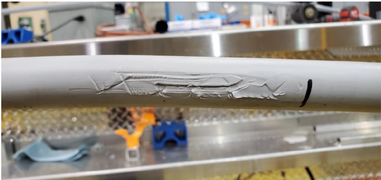
Figure 6-4: Hendrix HPI-35VTP-02 - Typical 397.5 kcmil (22 kV) AAC Conductor Condition after Slip Test
