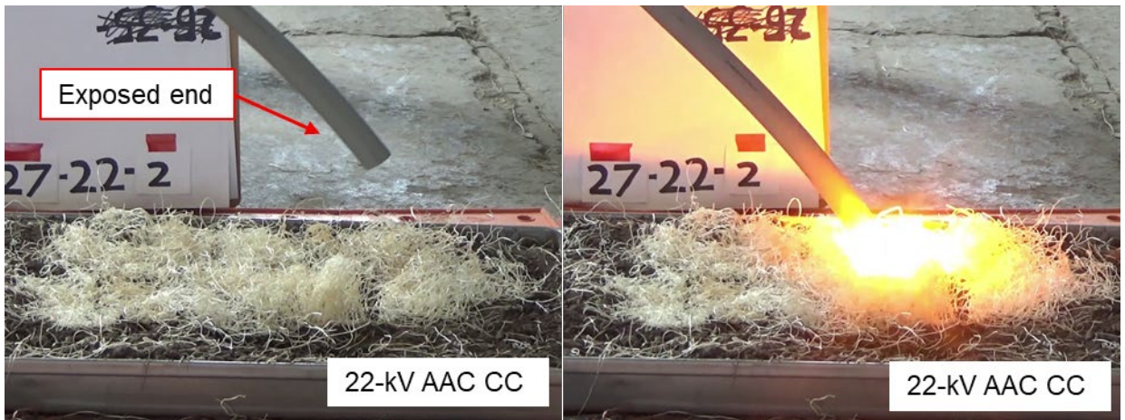
Figure B4. Simulated wire-down test of a 22-kV AAC CC with a broken end demonstrating the potential for ignition of the dry brush.
