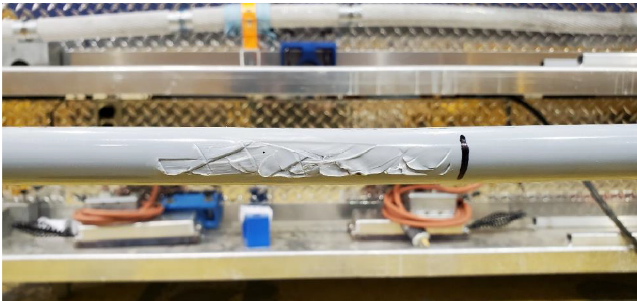
Figure 6-2: Hendrix HPI-35VTP-02 - Typical 1/0 AWG (17 kV) ACSR Conductor Condition after Slip Test
