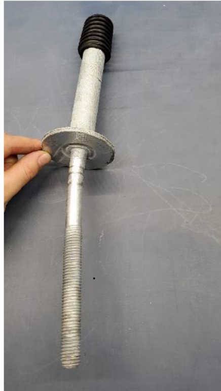
Figure 6-5: Hendrix HPI-35VTP-02 - Typical Bend in Insulator Pin after Slip Test
