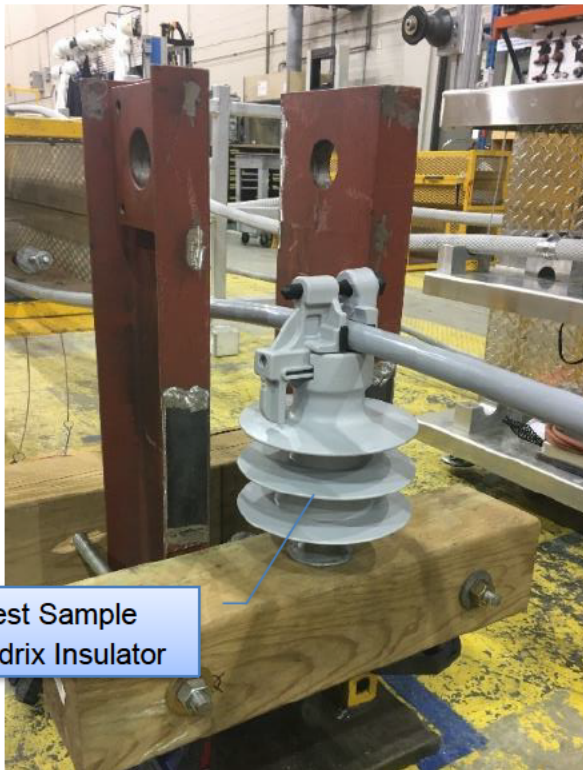
Figure 4-2: Clamp Slip Test Setup
