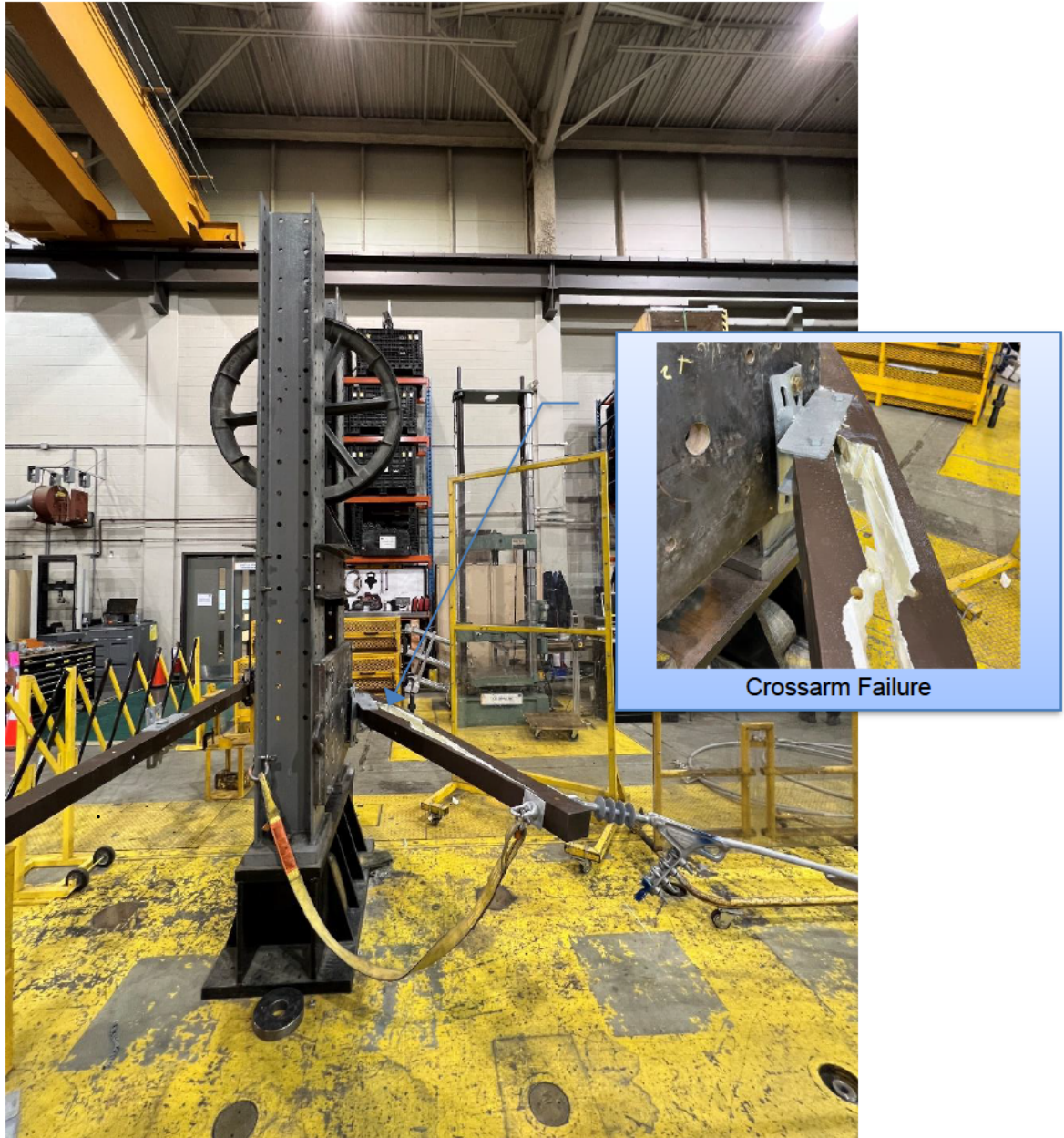
Figure 6-22: Sample 6.1 – Failure Location
