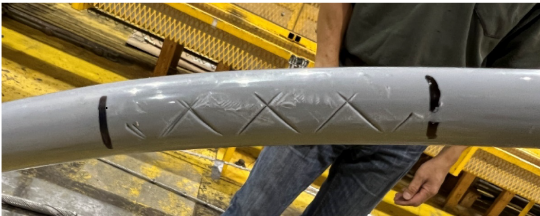
Figure 6-8: Sample 3.1.1 - 17 kV, 1/0 AWG ACSR Condition after Test
