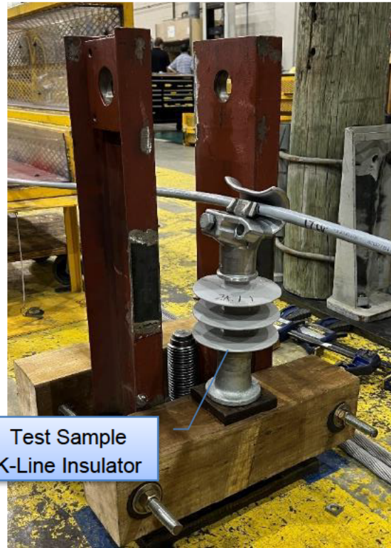
Figure 4-2: Clamp Slip Test Setup
