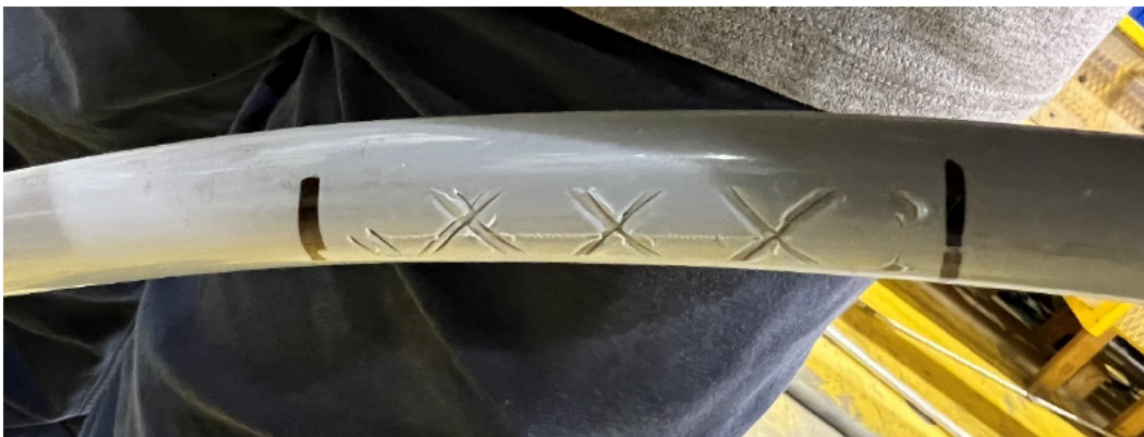
Figure 6-10: Sample 3.1.2 - 17 kV, 1/0 AWG ACSR Condition after Test
