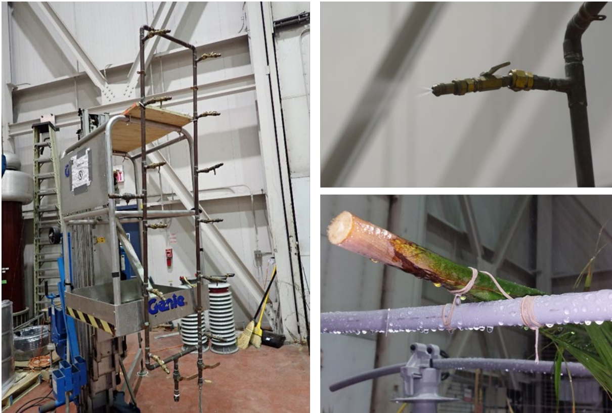
Figure A4. Wet test setup for phase-to-phase contact tests.
