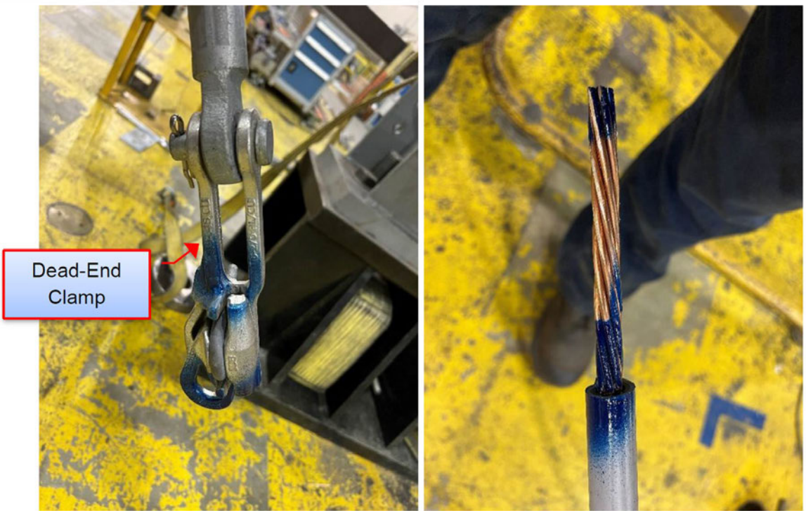
Figure E3. A representative post-test image showing pull-out of the conductor at the dead-end clamp attached to the insulator (north end). 2/0 CU with MPS ASO-398-1 NTP dead-end shown.
