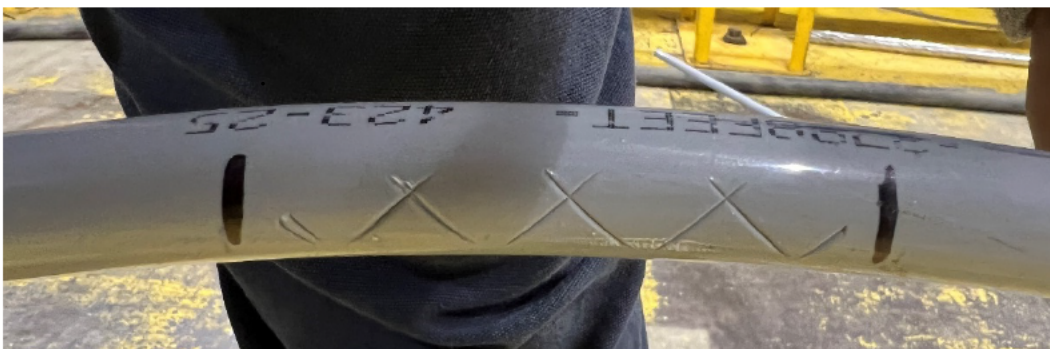
Figure 6-12: Sample 3.1.3 - 17 kV, 1/0 AWG ACSR Condition after Test
