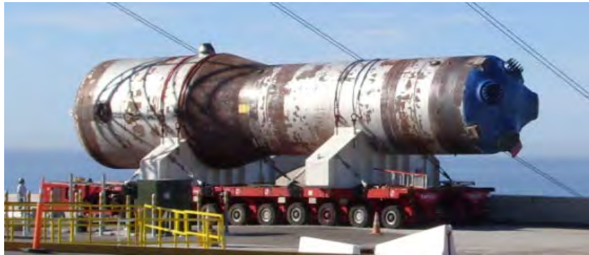
Steam Generator being transported to a specified storage area.
