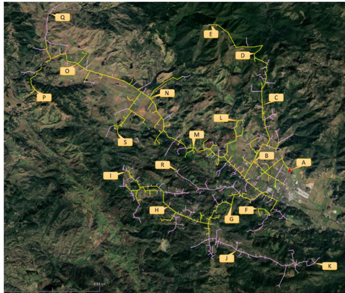
Figure 8. Feeder concept plan showing suggested RF data collection sites
