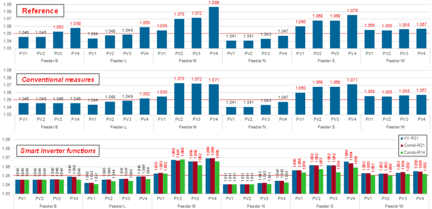
Figure 19: Maximum Secondary Overvoltage
