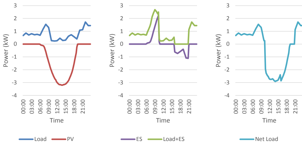
Figure 4-15 Example of Sufficient Solar Energy Storage Operation: Left: Original Load and Generation Profiles; Center: ES Profile and New Loadshape (Considering ES But Not PV); and Right: Net Household Load (With Load, ES, and PV Generation)
