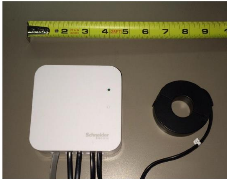
Figure B-1: Image of ZigBee® PV submeter, including Current Transformer (CT)
