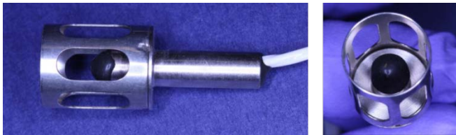
Figure 5-2 Ambient Temperature Sensor Inside the RTU
