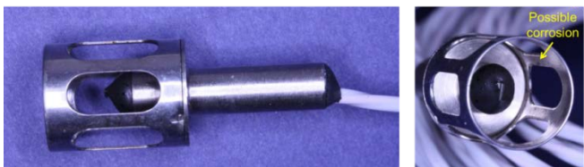
Figure 5-3 Ambient Temperature Sensor Inside the Data Concentrator
