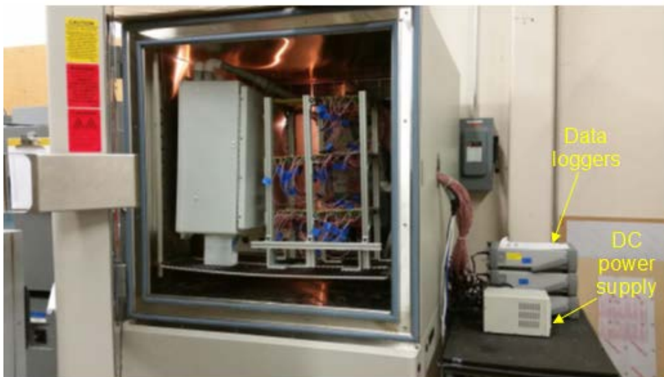
Figure 4-1 Environmental chambers used for accelerated lifecycle testing
