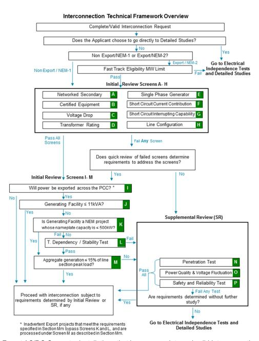
\* Non-Export AC/DC Converter installations that have a complete and valid Interconnection Request will be eligible to bypass screens B through D and F through M. If Generating Facility meets the conditions in Screen I below (Section G.1.i), skip Screens K, L and M.
