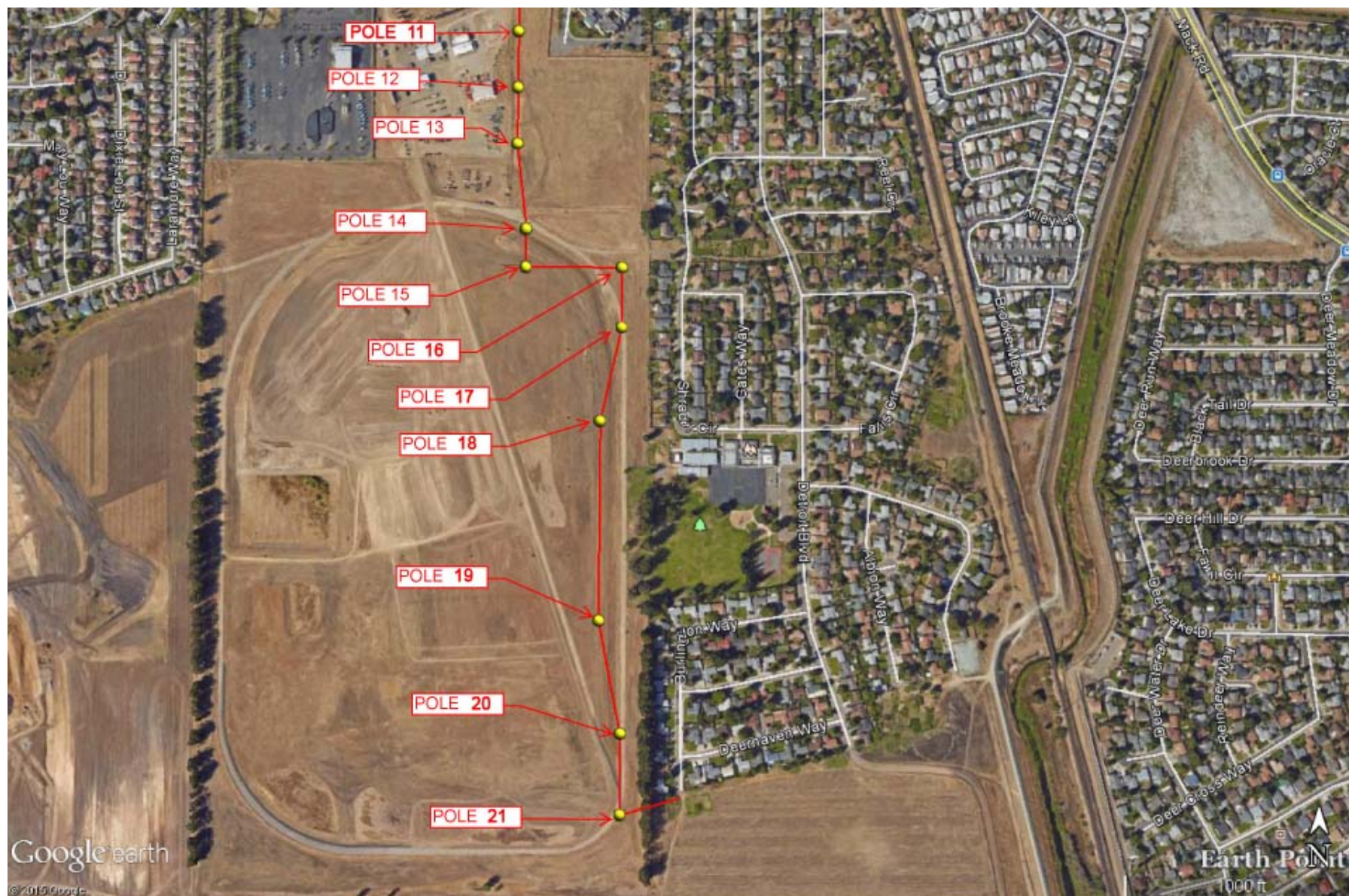
Figure 1-3b. 69KV Transmission Line Relocation – Southern Portion
