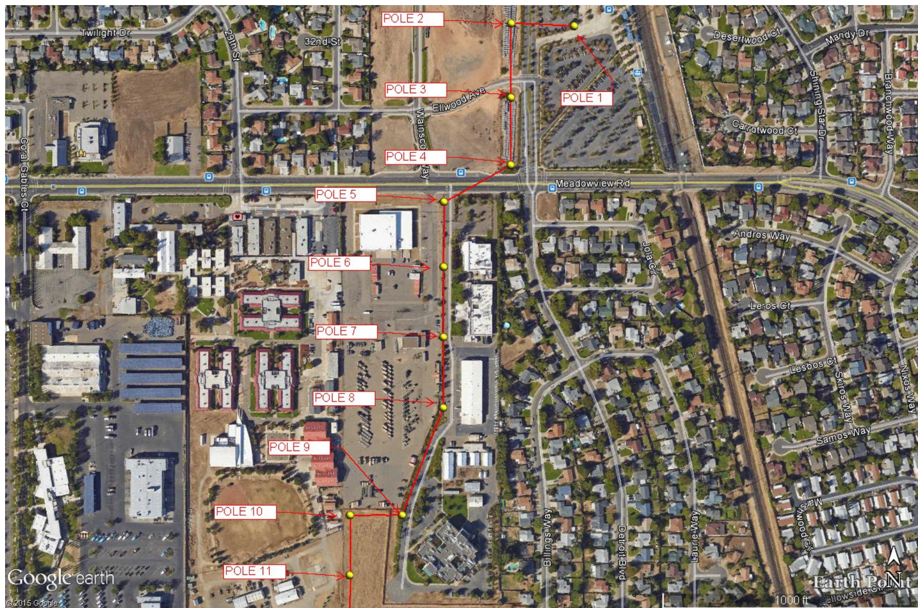
Figure 1-3a. 69kV Transmission Line Relocation – Northern Portion
