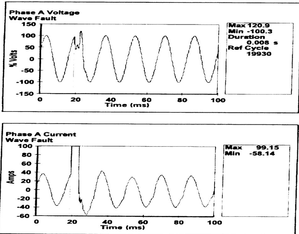
Figure 4 - Typical current-limiting fuse operation showing brief sag followed by peak arc voltage when fuse clears.
