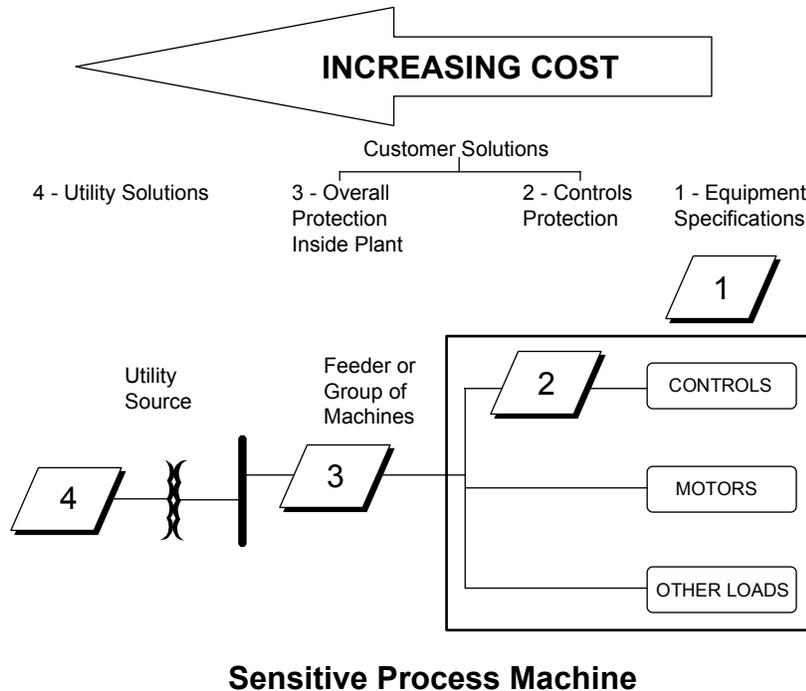
*Figure 8, Four Approaches for voltage sag ride-through.*
