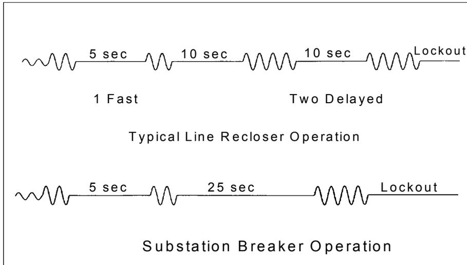
Figure 3. The most common reclosing sequences for line reclosers and substation breakers. In general, faults are to be cleared in less than 30 seconds
