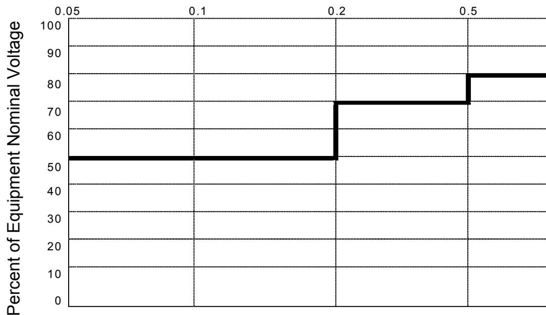
**Figure 7 - Required Semiconductor Equipment Voltage Sag Ride-Through Capability Curve**
