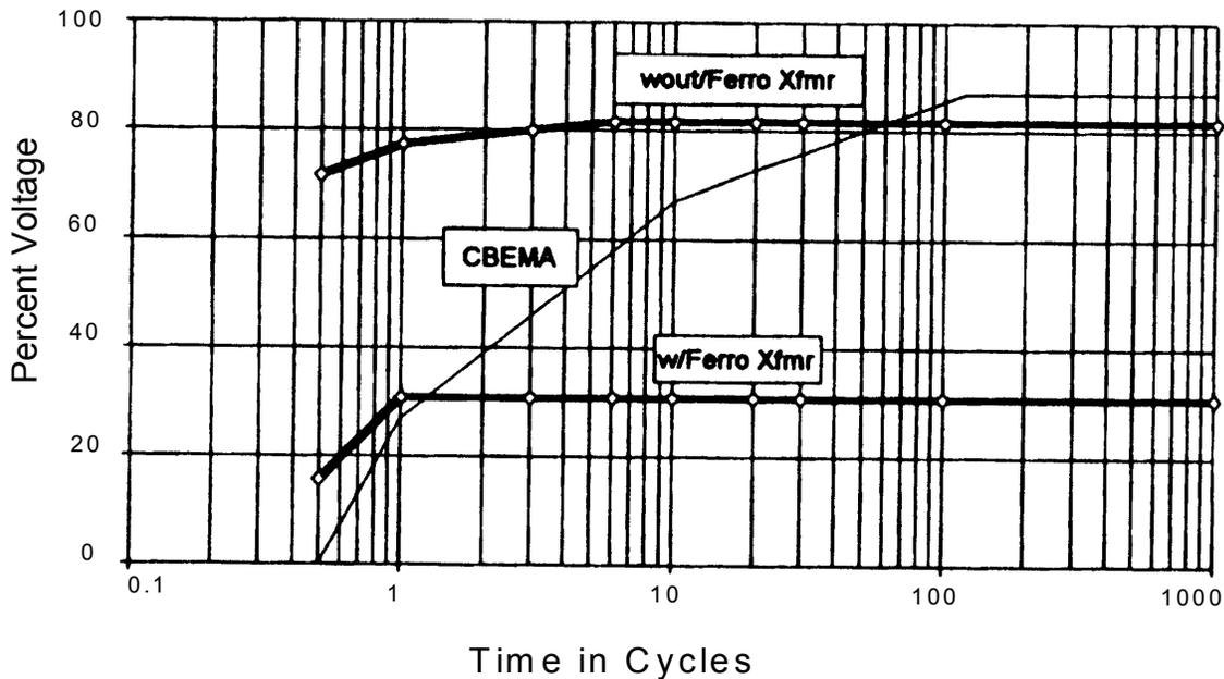
**Figure 10 - Voltage Sag Improvement with Ferroresonant Transformer**
