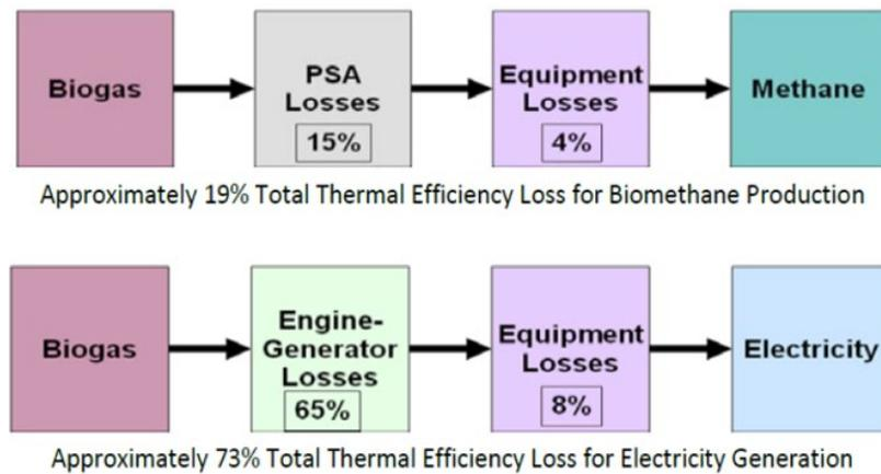
Figure 2 Biogas Utilization Thermal Efficiency Pathways (Krom, 2011)
