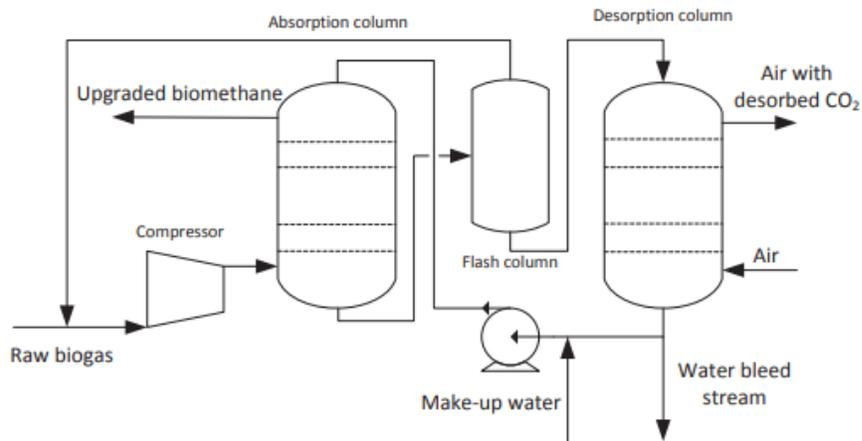
Figure 5 Typical water scrubbing process diagram (Bauer, 2012)
