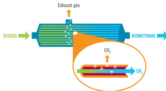
Figure 7 Membrane separation process (Fachverband Biogas e.V., 2017)
