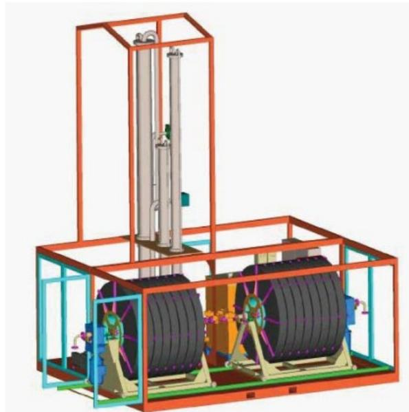
Figure 6 Rotary Coil Water Scrubber (Bauer, 2012)
