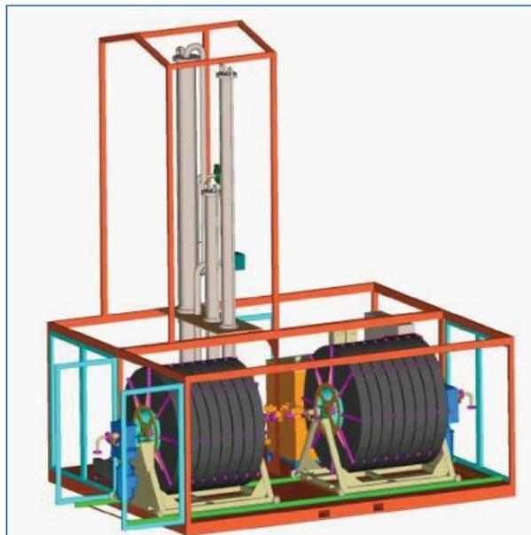
Figure 5 Illustration of a rotary coil water scrubber (Bauer, 2012)
