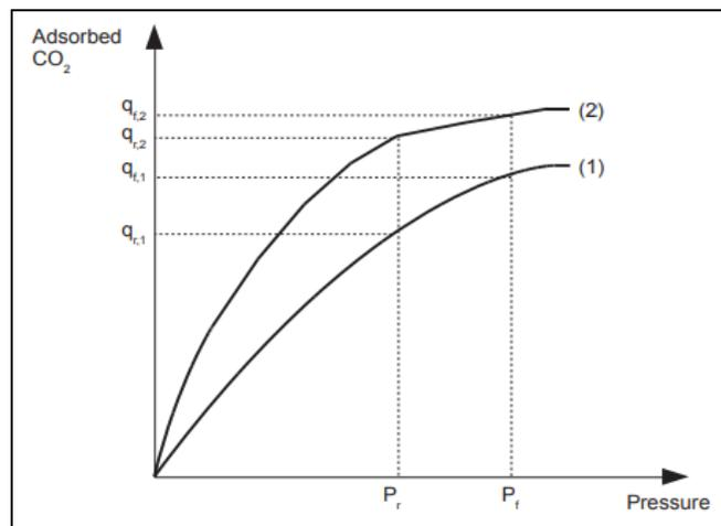
Figure 1 Graph showing the relationship between adsorbed CO<sub>2</sub> and pressure (Bauer, 2012)
