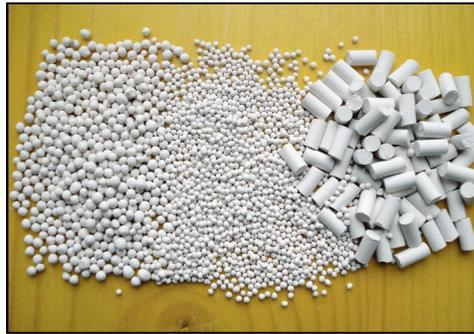
Figure 3 Picture of zeolites
