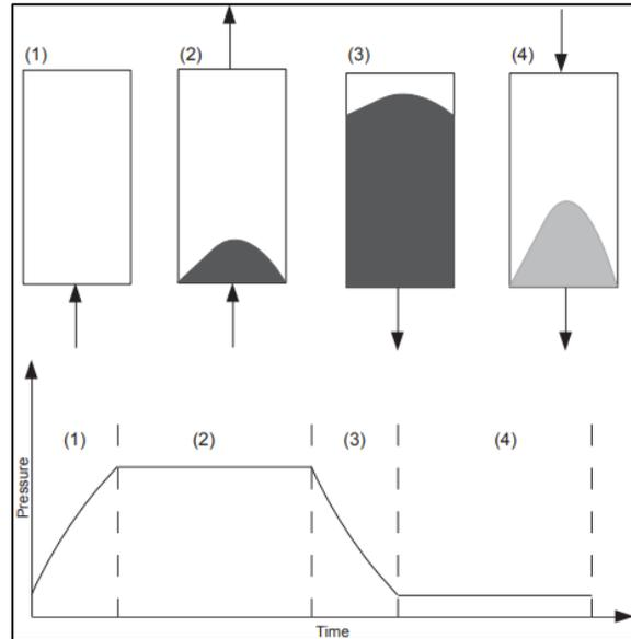
Figure 2 Illustration of the Skarstrom Cycle (Bauer, 2012)
