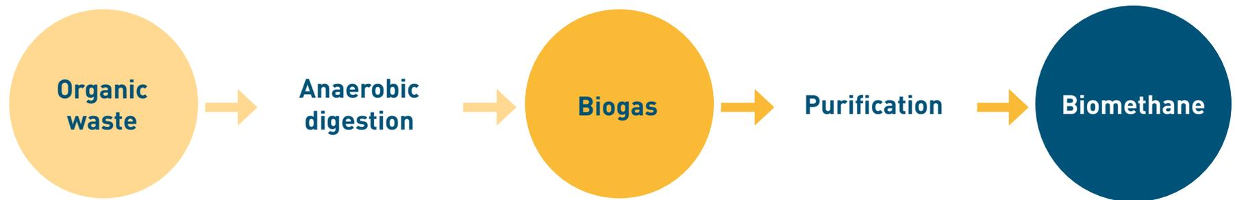
When this process is finished, you have pipeline-quality gas that is ready to enter the gas pipeline system or be burned for electricity generation. Both can be used in PG&E's service territory.
