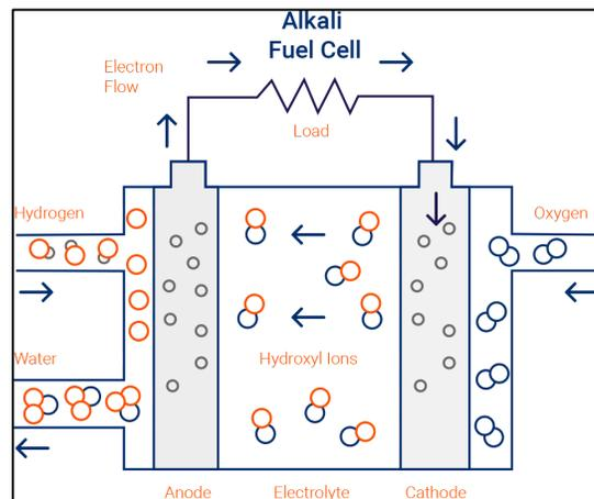
Figure 4 How Alkali Fuel Cells work
