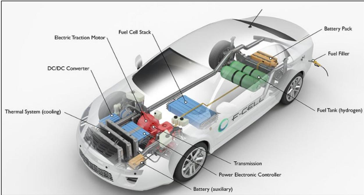
Figure 9 Illustration of a fuel cell vehicle (Energy Efficiency & Renewable Energy, 2018)
