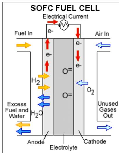
Figure 7 How a SOFC works
