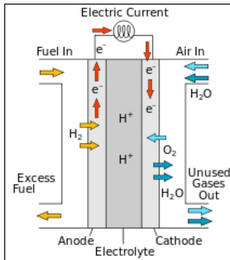
Figure 1 How a fuel cell works (Barone, 2018)
