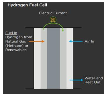
Figure 8 How a hydrogen fuel cell works
