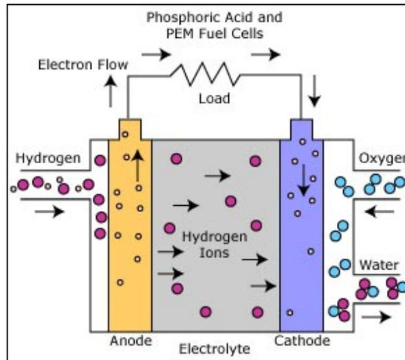
Figure 5 How PAFC work
