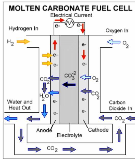
Figure 6 How a Molten Carbonate Fuel Cell works
