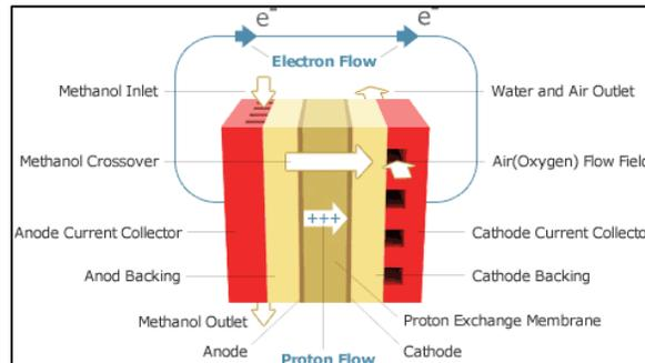
Figure 3 How DMFC works
