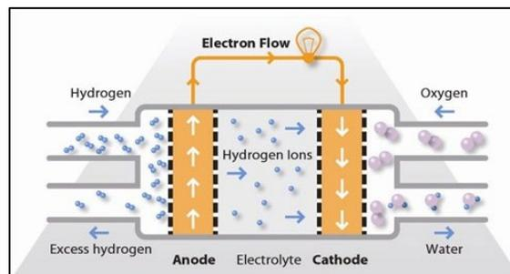
Figure 2 How PEMFC works
