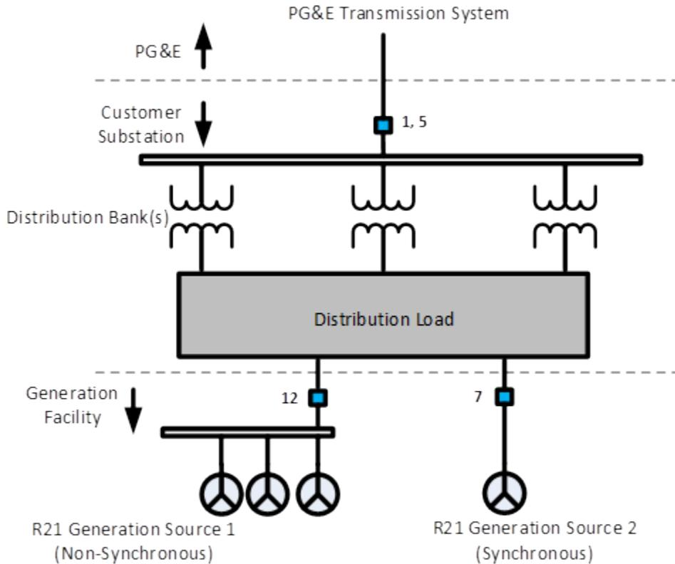
**Figure 2.1-C - Example Rule 21 Generator Telemeter Points**
