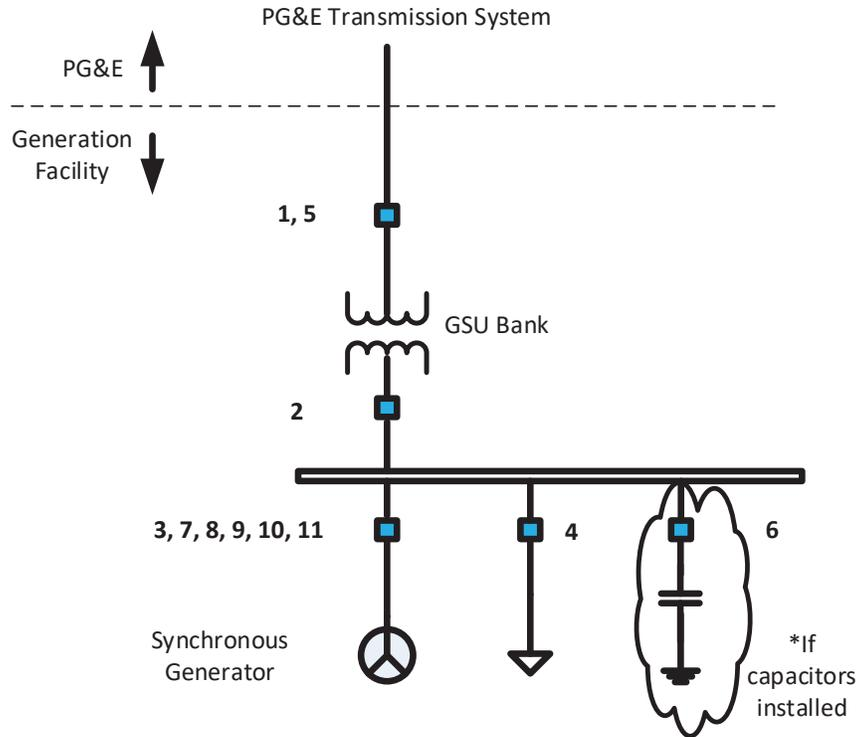
**Figure 2.1-A** - Example Synchronous Generator Telemeter Points
