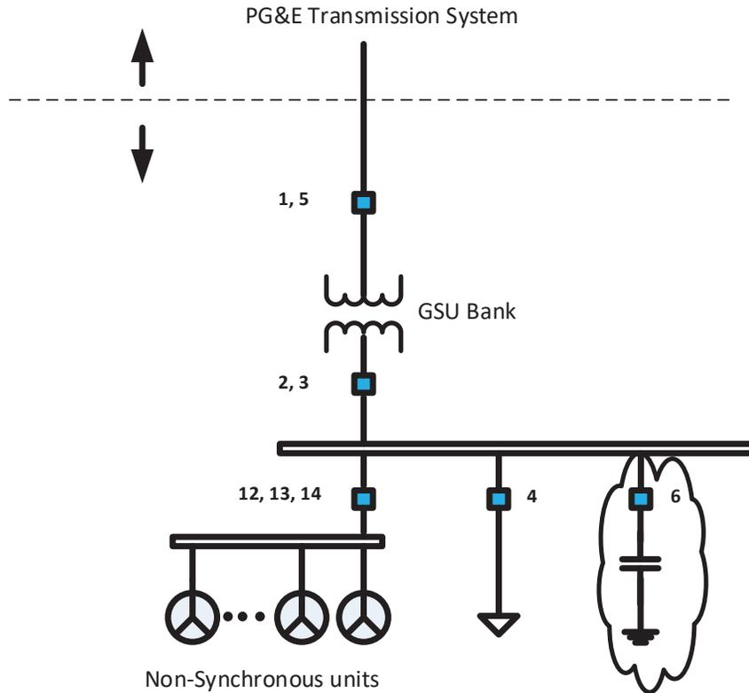
**Figure 2.1-B** - Example Non-Synchronous Generator Telemeter Points
