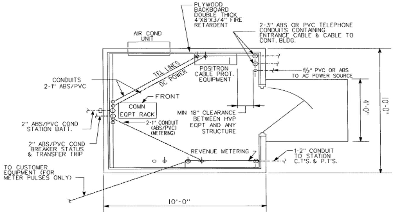
NOTE: RTU AND TRANSFER TRIP EQUIPMENT TO BE MOUNTED IN THE COMMUNICATIONS RACK
