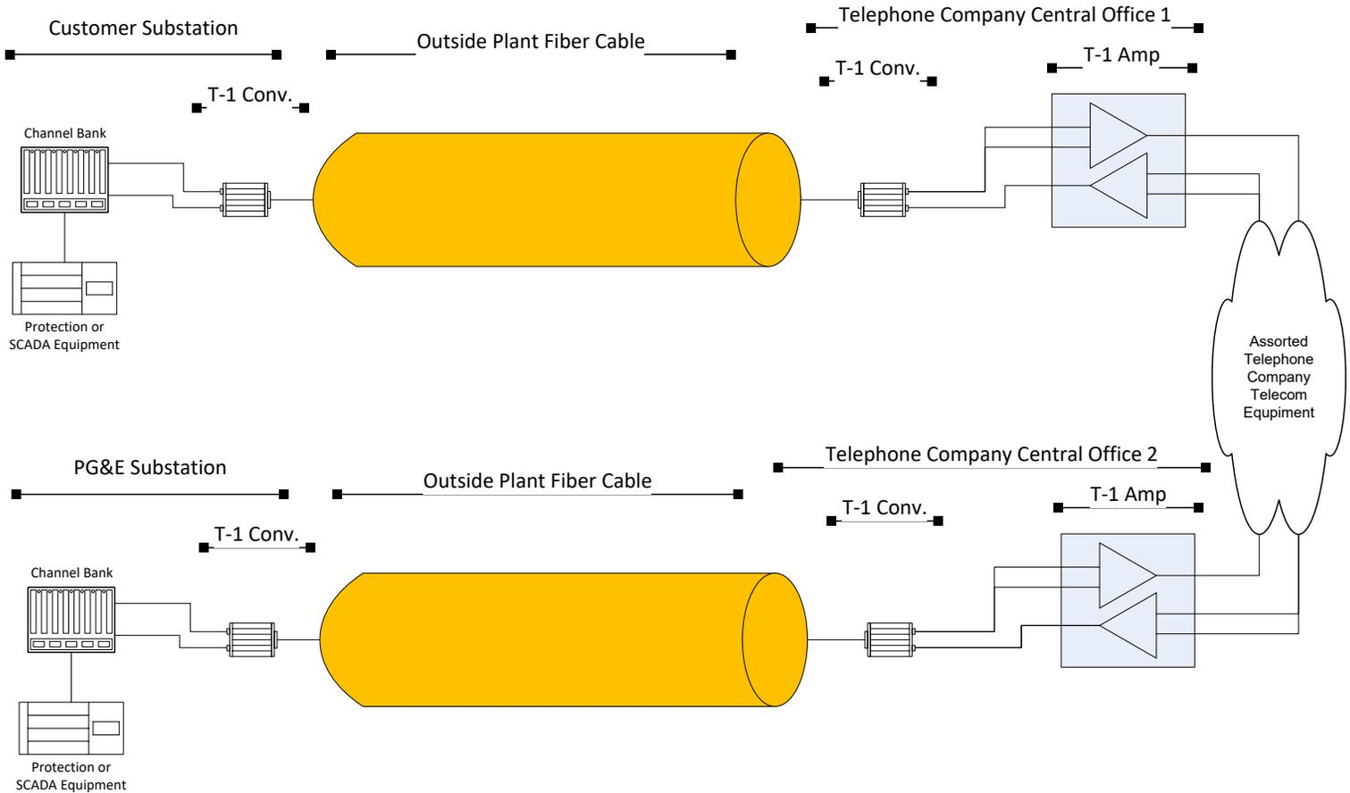
Protection Circuit Over All Fiber Between Substations
