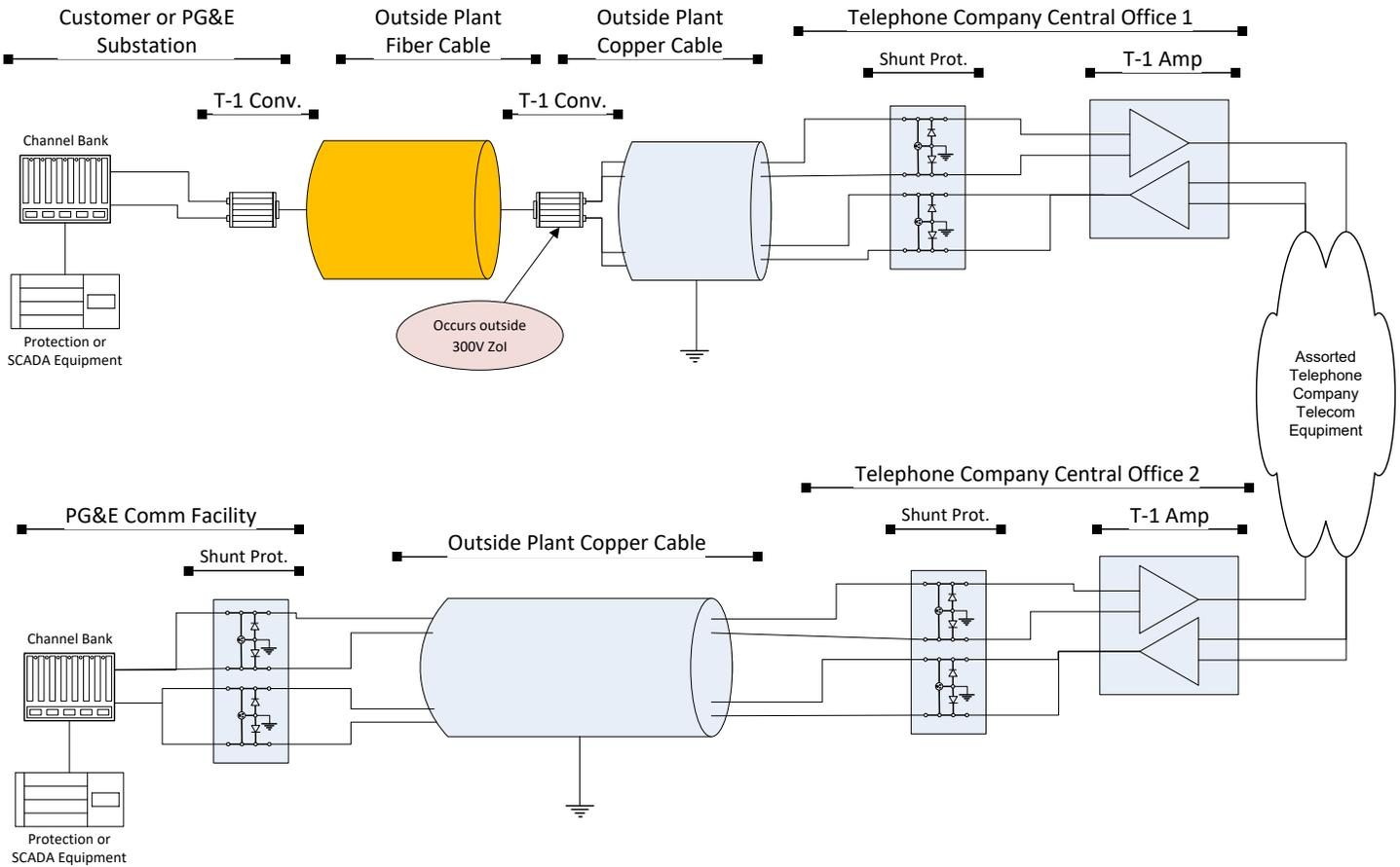
Protection Circuit Over Hybrid/Copper Facilities DTT Receiver programmed to trip the generator off line for a communication fail alarm on the Third Party Provided Telco lease line.
