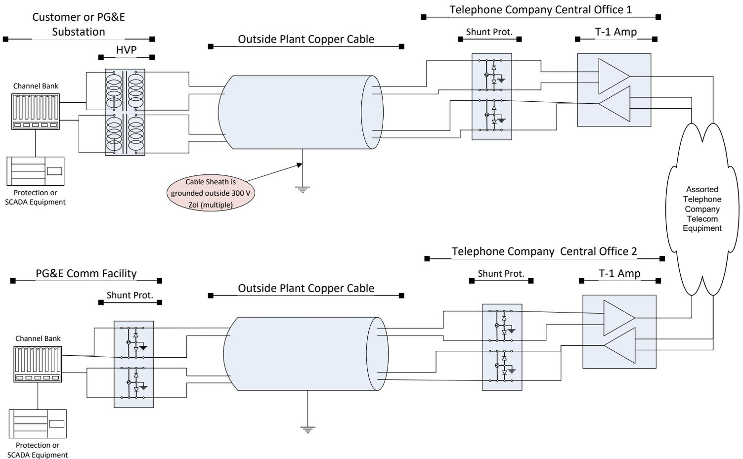
Protection Circuit Over Copper Facilities DTT Receiver programmed to trip the generator off line for a communication fail alarm on the Third Party Provided Telco lease line.
