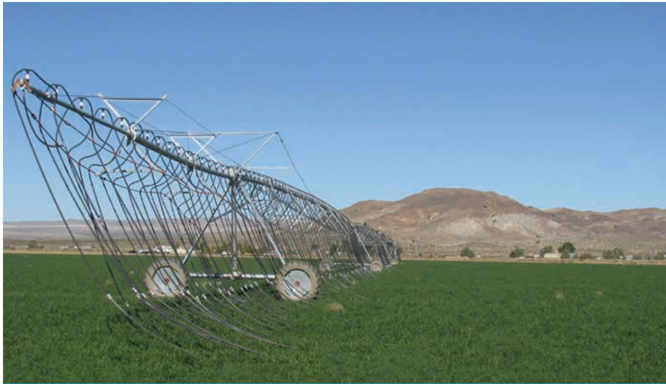
Drag-and-drip technology conserves water by reducing evaporation.
