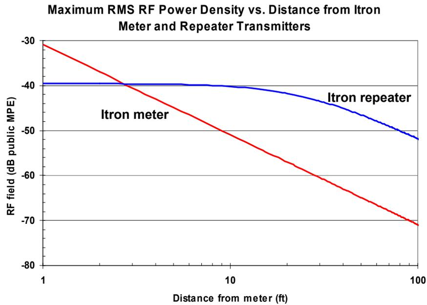
**Figure 7.** RMS RF field for the Itron meter and repeater transmitter vs. distance expressed as decibels relative to the FCC MPE value. 0 dB is equal to the MPE.
