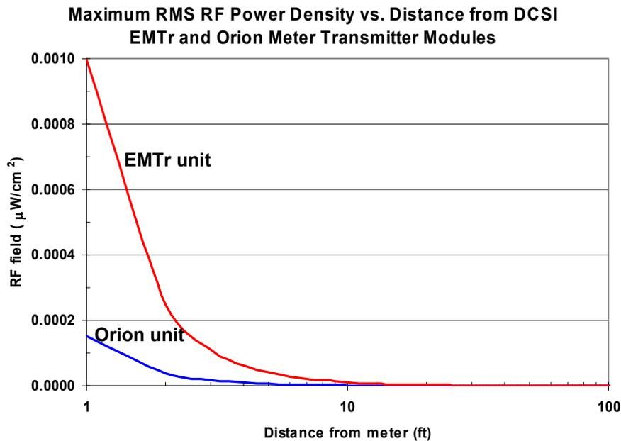
**Figure 4.** RMS RF field for the DCSI EMTr and Orion meter transmitter modules vs. distance expressed as power density in microwatts per square centimeter ( $\mu\text{W}/\text{cm}^2$ ). The public MPE is equal to  $601 \mu\text{W}/\text{cm}^2$  for the DCSI frequency.
