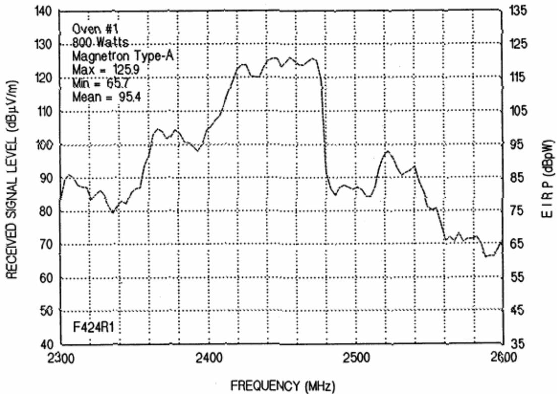
**Figure 9.** Peak electric field strength at 3 meters vs. frequency plot of microwave oven signals from NTIA report (Gawthrop et. al, 1994). The maximum signal strength measured in this example was equivalent to 1.972 V/m or 1.03  $\mu$ W/cm<sup>2</sup>.
