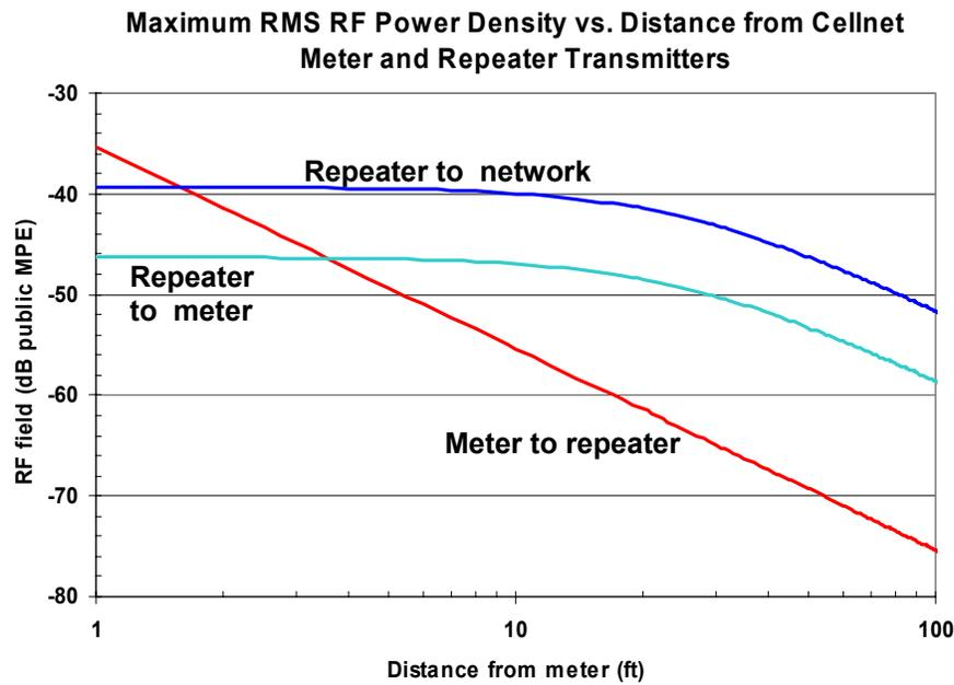
**Figure 1.** RMS RF field for the Cellnet meter and repeater modules vs. distance expressed as decibels relative to the FCC MPE value. 0 dB is equal to the MPE.
