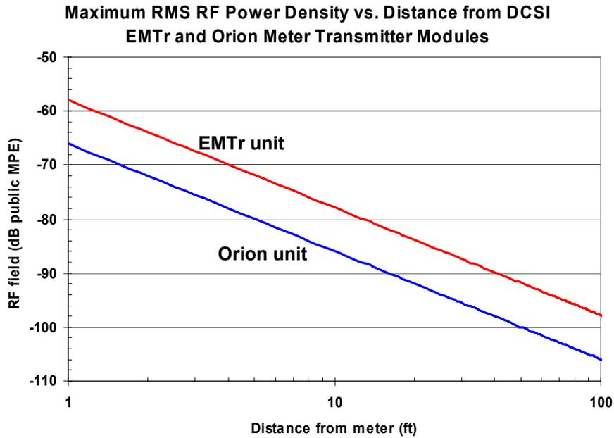
**Figure 3.** RMS RF field for the DCSI EMTr and Orion meter transmitter modules vs. distance expressed as decibels relative to the FCC MPE value. 0 dB is equal to the MPE.
