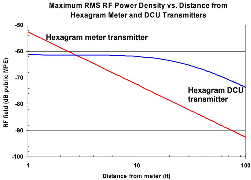
**Figure 5.** RMS RF field for the Hexagram meter and DCU transmitters vs. distance expressed as decibels relative to the FCC MPE value. 0 dB is equal to the MPE.
