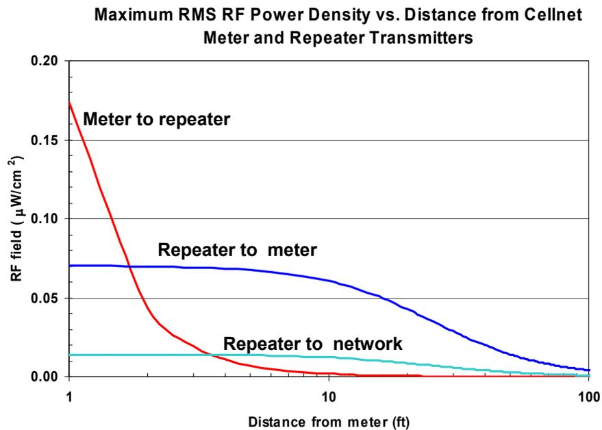
**Figure 2.** RMS RF field for the Cellnet meter and repeater modules vs. distance expressed as power density in microwatts per square centimeter ( $\mu\text{W}/\text{cm}^2$ ). The public MPE is equal to  $601 \mu\text{W}/\text{cm}^2$  for the Cellnet frequency.
