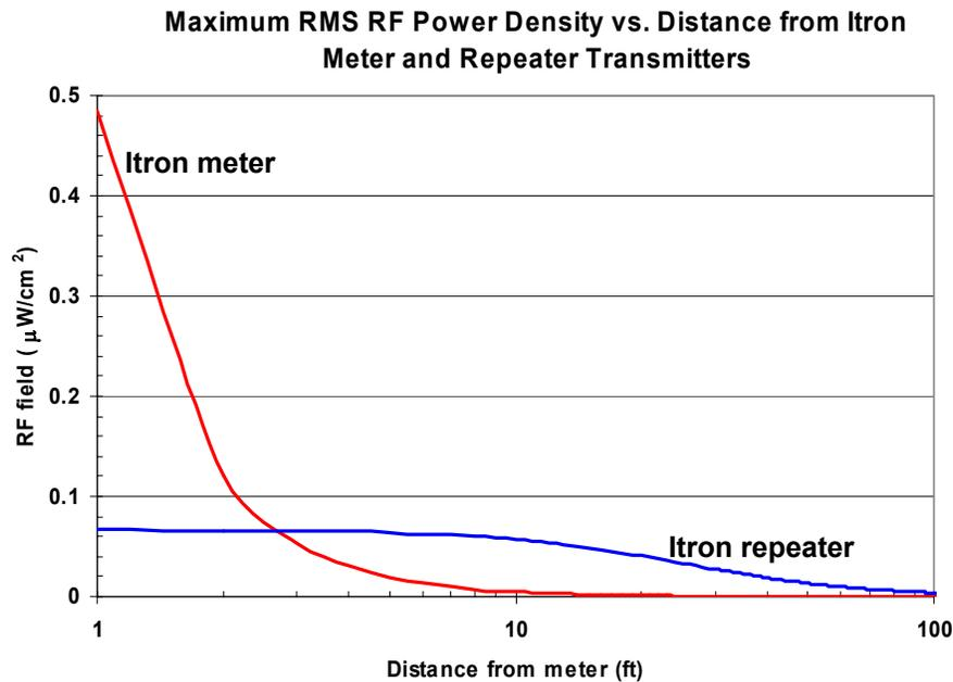
**Figure 8.** RMS RF field for the Itron meter module and repeater transmitter vs. distance expressed as power density in microwatts per square centimeter ( $\mu\text{W}/\text{cm}^2$ ). The public MPE is equal to  $601 \mu\text{W}/\text{cm}^2$  for the Itron frequency.
