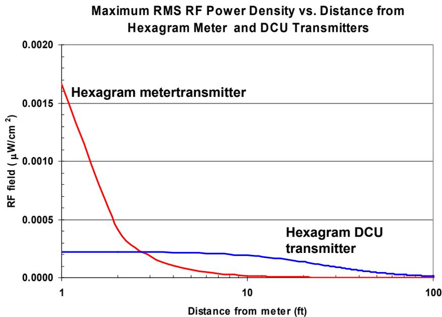
**Figure 6.** RMS RF field for the Hexagram meter and DCU transmitters vs. distance expressed as power density in microwatts per square centimeter ( $\mu\text{W}/\text{cm}^2$ ). The public MPE is equal to  $300 \mu\text{W}/\text{cm}^2$  for the Hexagram frequency.
