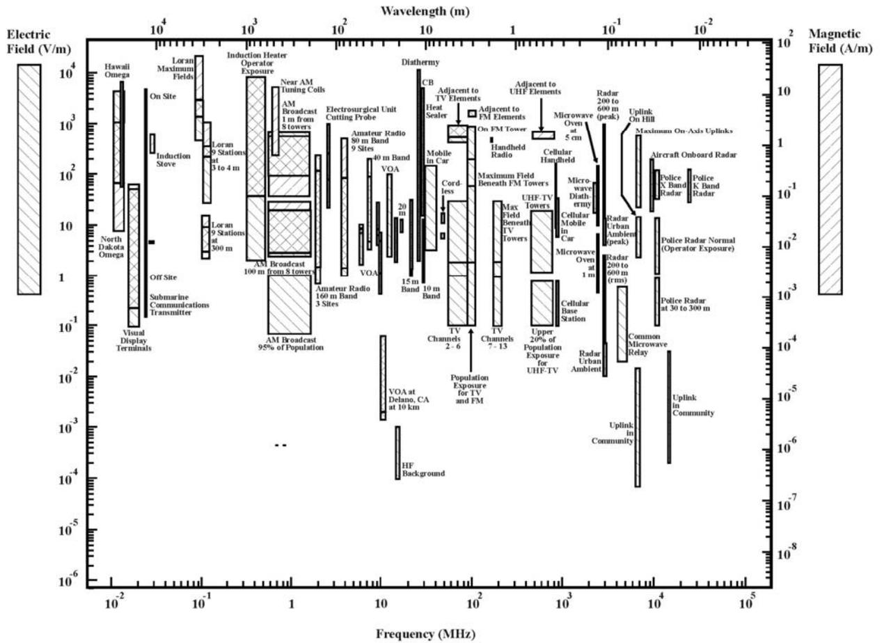
Summary of Measured Radio Frequency Levels in the General and Work Environment (U.S. EPA - 1997)
