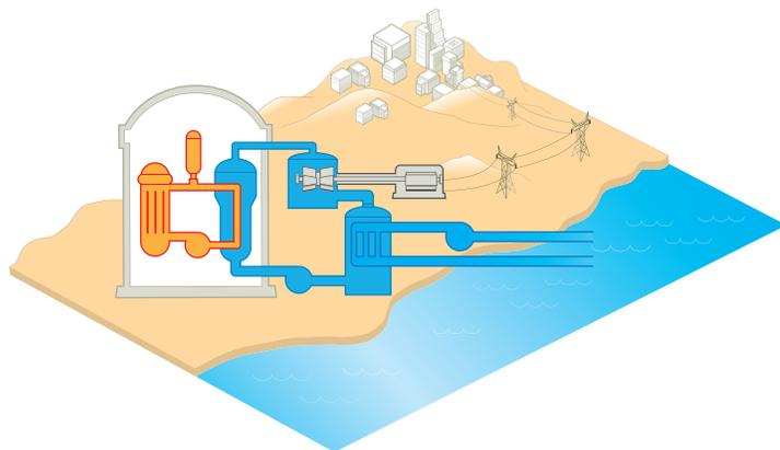
allowing the water to reach over 600 degrees Fahrenheit and 2,200 pounds per square inch of pressure. This water is radioactive so it is enclosed inside the protective reactor containment dome.
