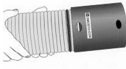
Figure 23 Key-Lock™ Couplers Insertion
