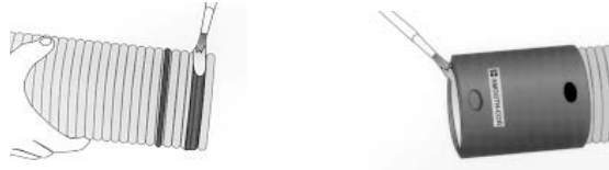
Figure 22 Key-Lock™ Couplers Lubricant Application
