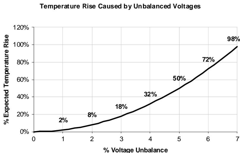
**Figure 1: Percent Temperature Rise Due to Voltage Unbalance**
