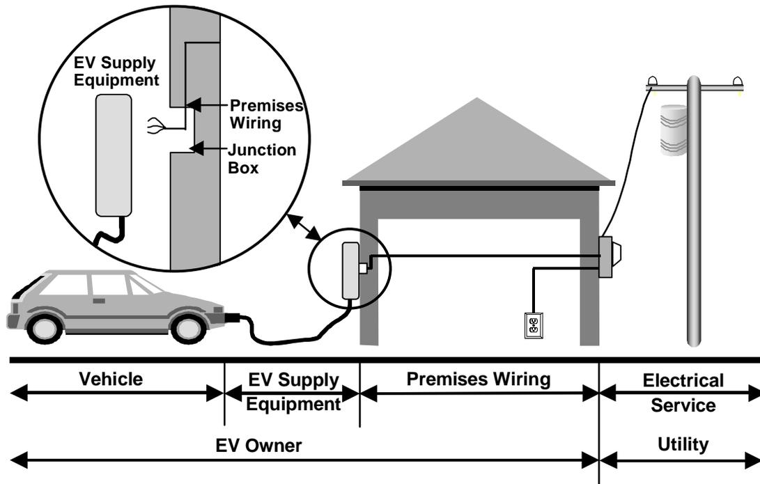
PG&E owns, installs, and maintains the electric service to the customer meter, in addition to providing electricity. For residences, PG&E offers special EV time-of-use (TOU) rates that provide incentives to charge EVs off-peak. To take advantage of some of the special rates, the EV owner may want install a second meter for the EVSE circuit (see Chapter 2E, *PG&E EV Rates*, for more information).
