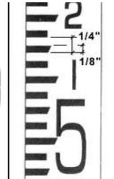
*Figure 10: Leveling rod detail*
