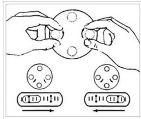
*Figure 7. "The Golden Rule for quick and simple leveling is THUMBS IN, THUMBS OUT. Turn BOTH screws equally and simultaneously. Practice will help you get the feel of the screws and the movement of the bubble. It will also help to remember that the direction your left thumb moves is the direction the bubble will move." Drawn images shown for Step 2 are from the David White Owner's Manual #8814-802.*
