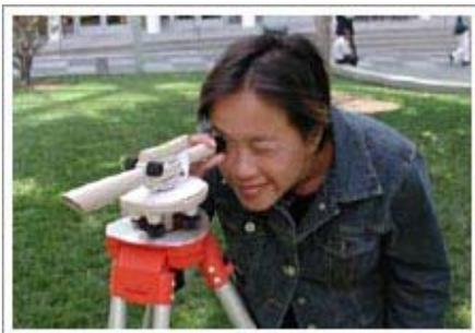
*Figure 11: Look through the telescopic sight eyepiece at the measuring rod.*
