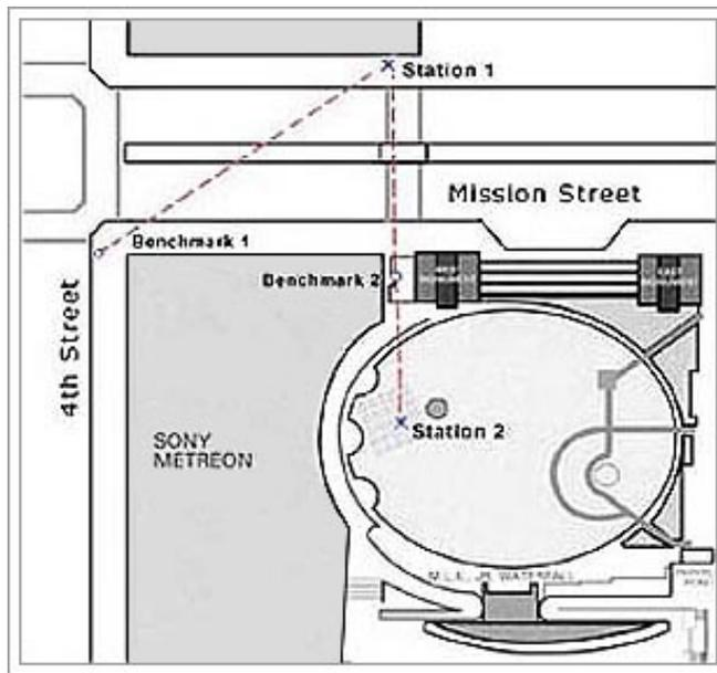
Figure 4: Plan for projecting the benchmark elevation into the site
