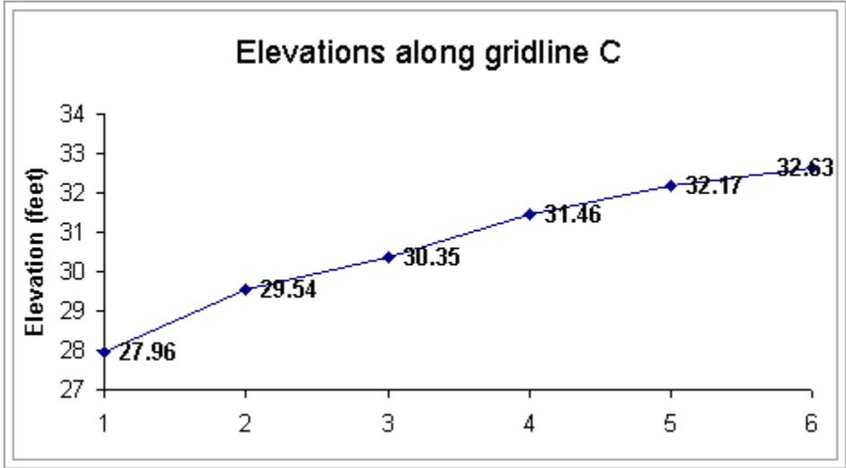
**Figure 18:** Section along gridline C. The distance between each grid line is 10'-0".
