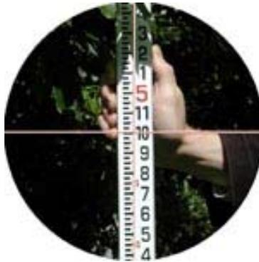
*Figure 9. Reading the leveling rod through the Level.*
