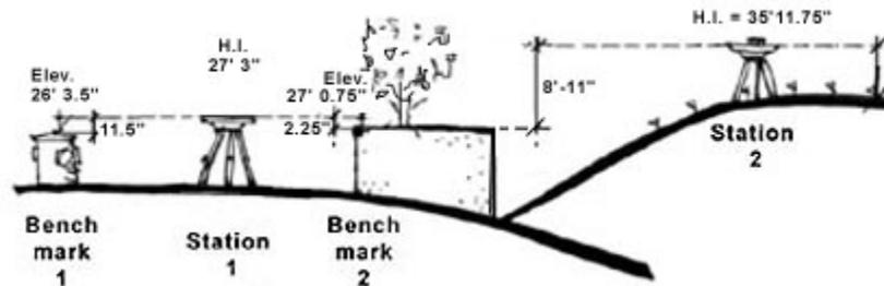
Figure 14: Benchmark and Station Section Diagram of plan in Fig. 10
