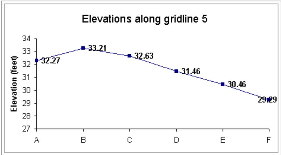
**Figure 17:** Section along gridline 5. The distance between each grid line is 10'-0".
