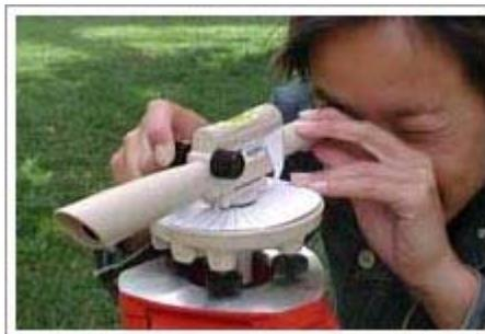
*Figure 12: Fine-tuning the focus by turning knobs*
