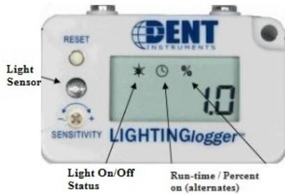
Figure 1: Dent LIGHTINGlogger
