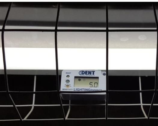
Figure 2: LIGHTINGlogger in lighting fixture
