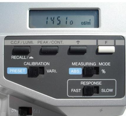
**Figure 2: Control panel and LCD display, displaying luminance reading.**
