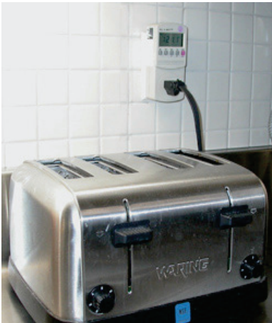
Figure 1: Kill-A-Watt meter monitoring energy use of an appliance
