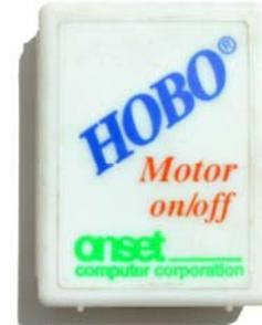
Figure 1: Hobo Motor on/off logger
