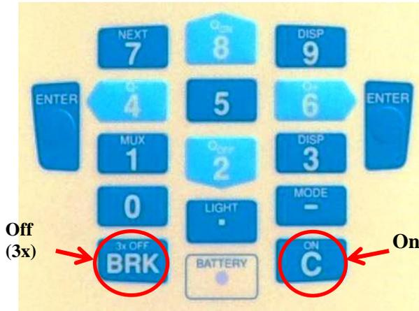
**Figure 5** Turn meter on and off (UM10.1 p61).
