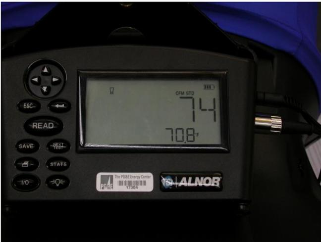
Figure 8. CFM and temperature display
