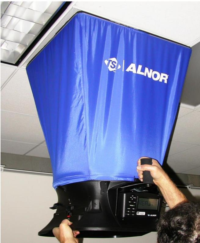
Figure 5. EBT721 in contact with register
