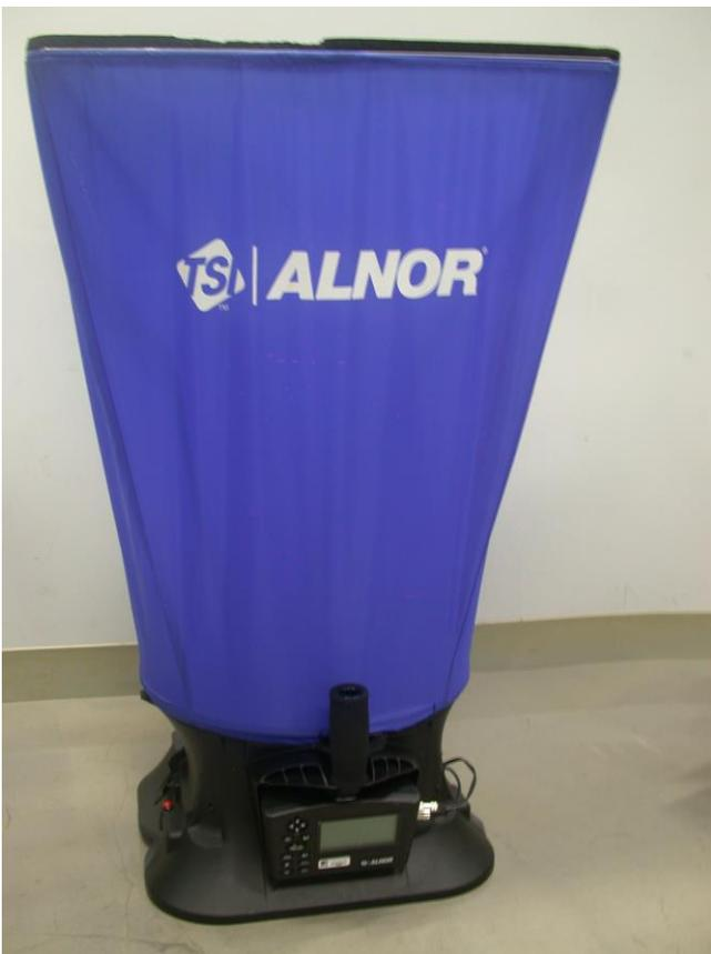
Figure 1. Alnor EBT721 Balometer
