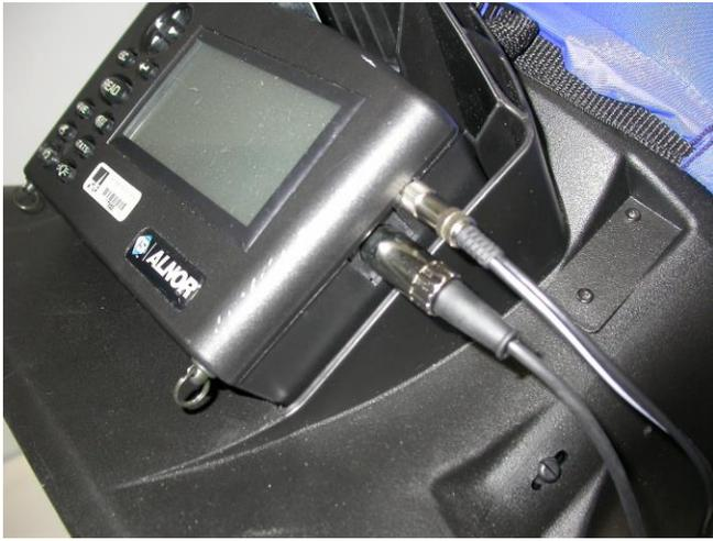
Figure 2. Temperature and back pressure cables connecting into meter
