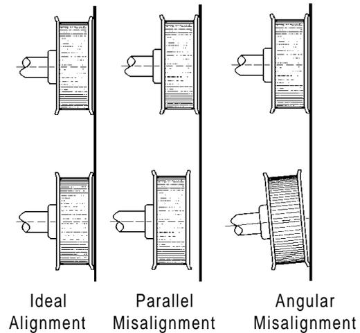
Figure 3: Typical misalignments of sheaves (Source: Fuchs)\*
