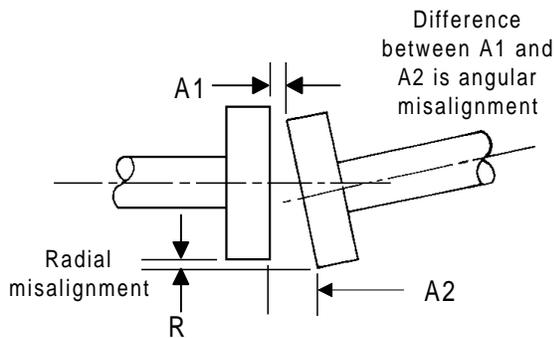
Figure 2: Typical misalignment of motor coupling (Source: Fuchs)\*
