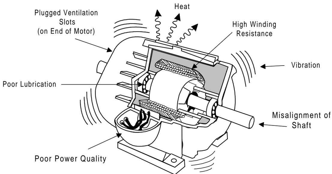
Figure 1: Sources of Potential Motor Efficiency Losses that can be Avoided with Proper Maintenance (Reprinted with permission. Copyright 1992 by Dranetz Technologies, Inc. All rights reserved.)
