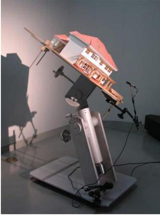
Model undergoing heliodon testing.
