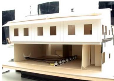
(b) The façade was removed so that the photocells could be easily moved.
