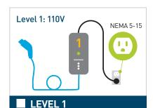
Charging stations usually require no upgrade to your service panel and are equivalent to plugging an EV into a standard household 110-volt wall outlet. Manufacturers typically include a Level 1 cord set with EV purchase.
