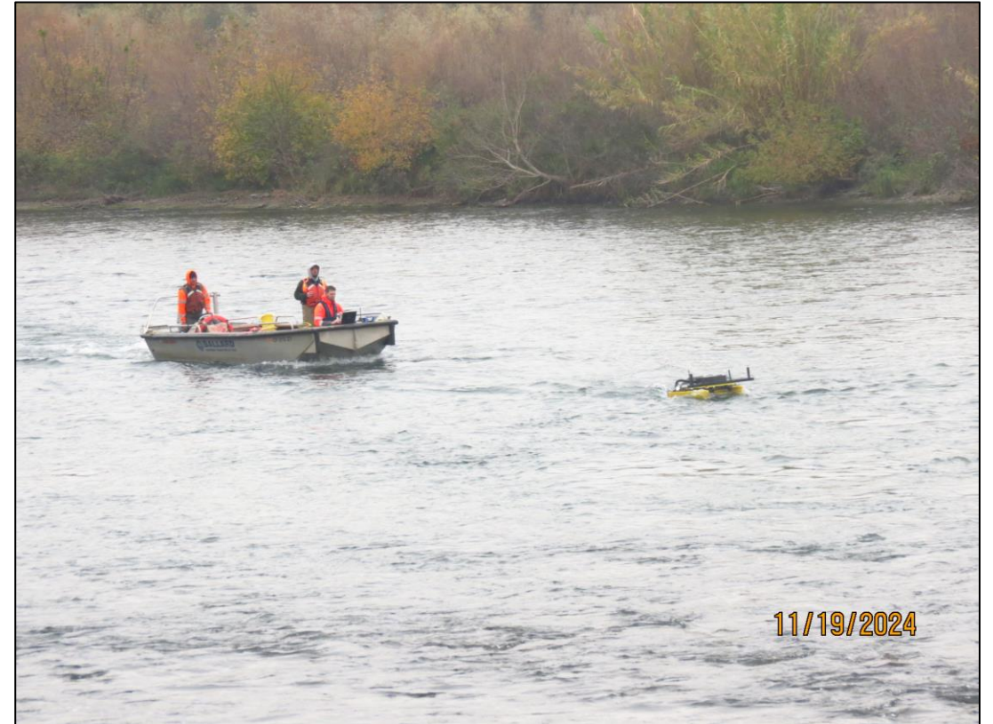
Non-intrusive survey of pipeline integrity at a Sacramento River Crossing Site
