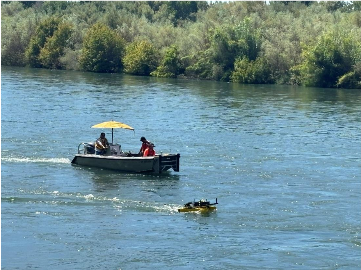
Figure 9: CMI non-intrusive survey of transmission pipeline integrity on boat platform at a Sacramento River Crossing site in Red Bluff.
