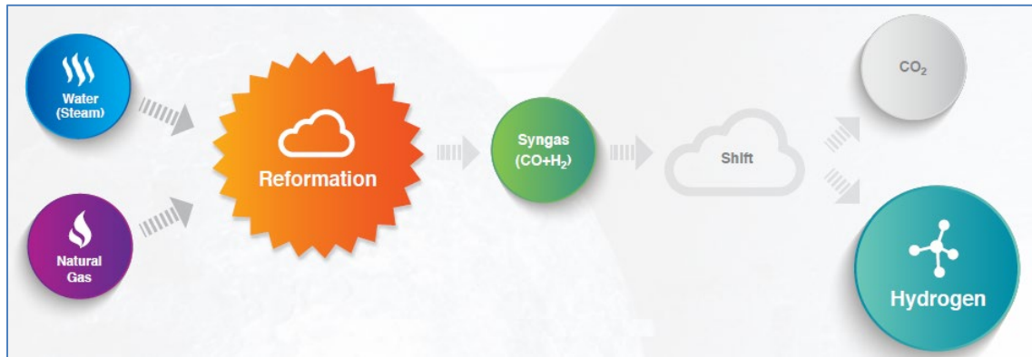
Figure 3 Steam Methane Reforming Path (PG&E R&D and Innovation, 2018)
