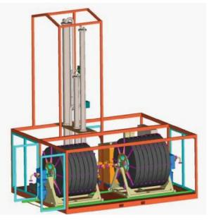
Figure 6 Rotary Coil Water Scrubber (Bauer, 2012)
