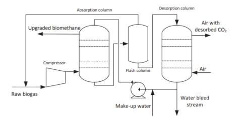
Figure 5 Typical water scrubbing process diagram (Bauer, 2012)
