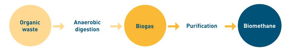
When this process is finished, you have pipeline-quality gas that is ready to enter the gas pipeline system or be burned for electricity generation. Both can be used in PG&E's service territory.
