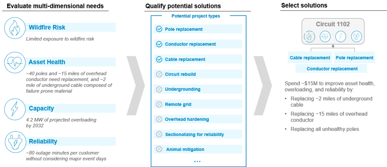
Figure 6. Circuit Needs to Consider When Bundling Work
