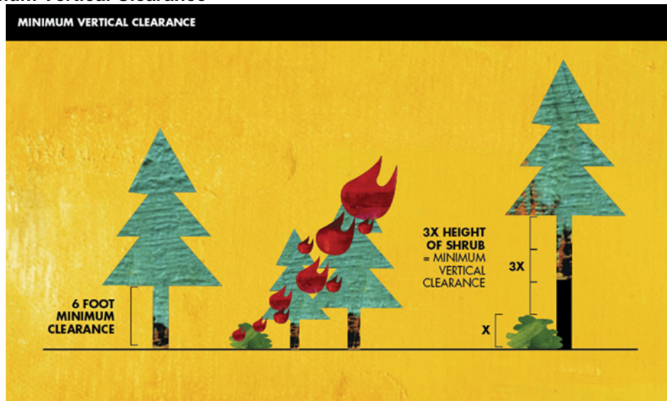
Figure 2, Minimum Vertical Clearance
