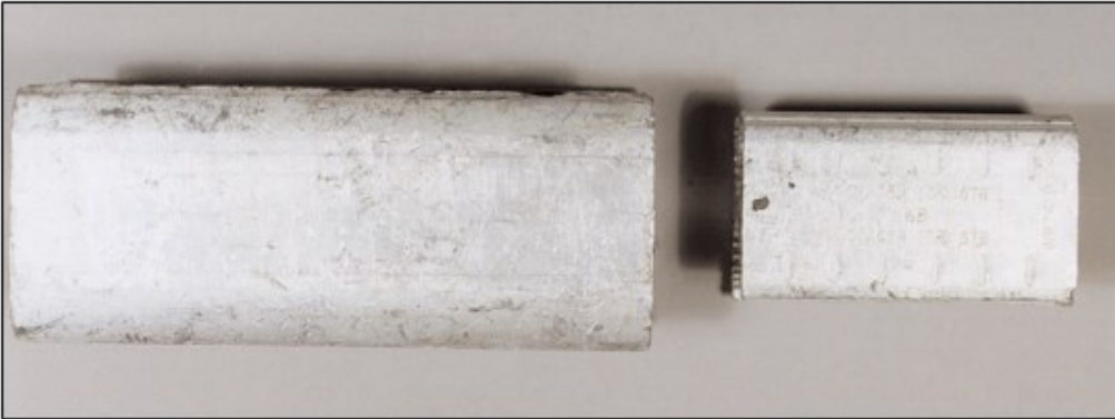
Figure B-72: H-Type Compression Connector (Not Compressed)
