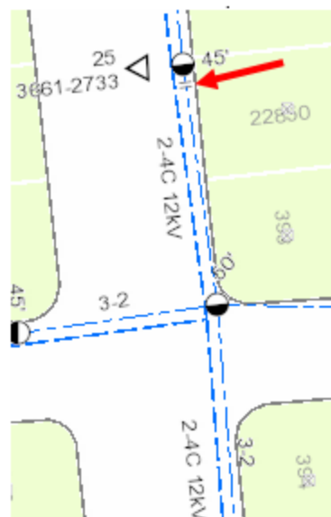
OH Transformers separated by bobs are ok
