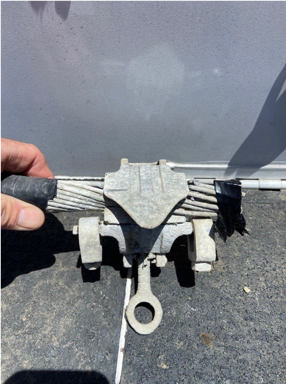
Figure 4 Chance clamp that was removed, side one. Photo taken by troubleshooter on June 2, 2024.
