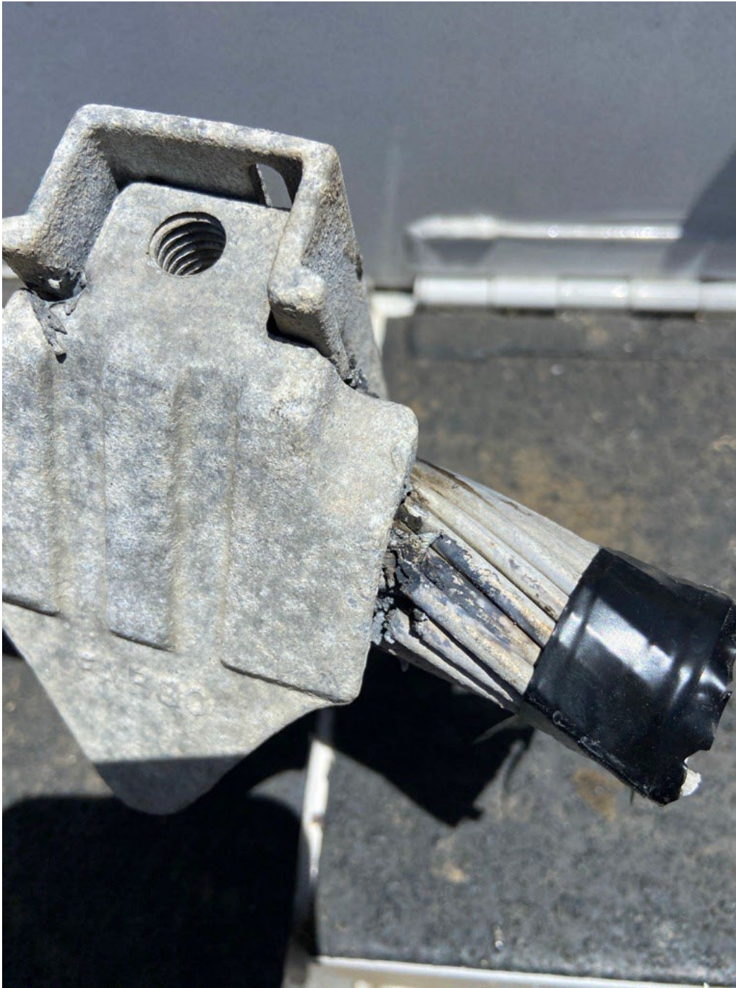
Figure 5 Chance clamp that was removed, side two. Photo taken by troubleshooter on June 2, 2024.
