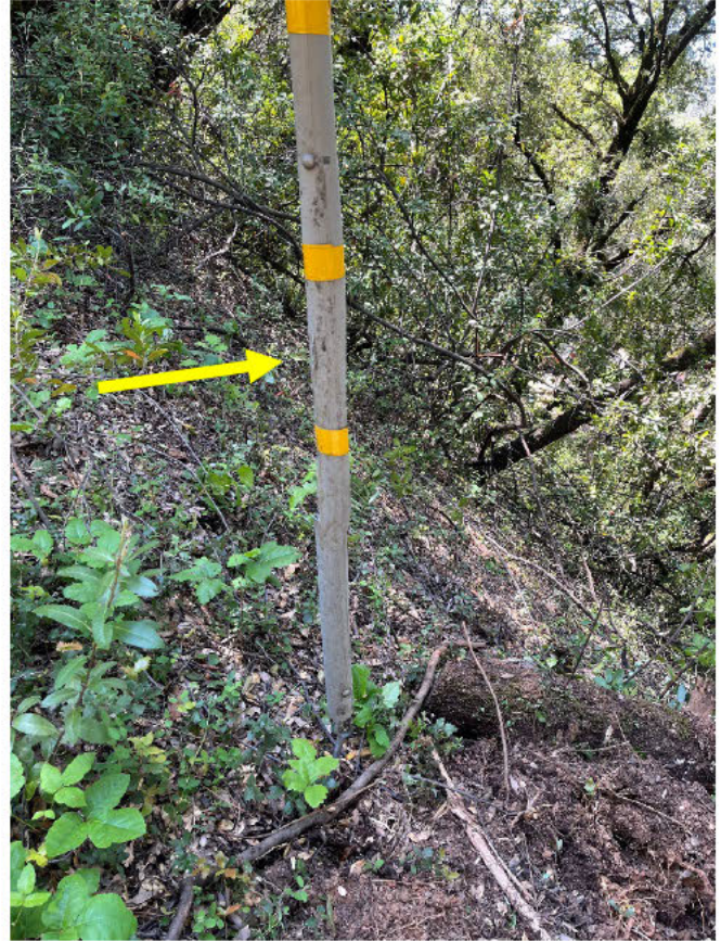
Figure 5 Guy wire from Pole #3 with visible damage and breakage on the plastic shell. Photo taken by ignition investigator on April 22, 2024.
