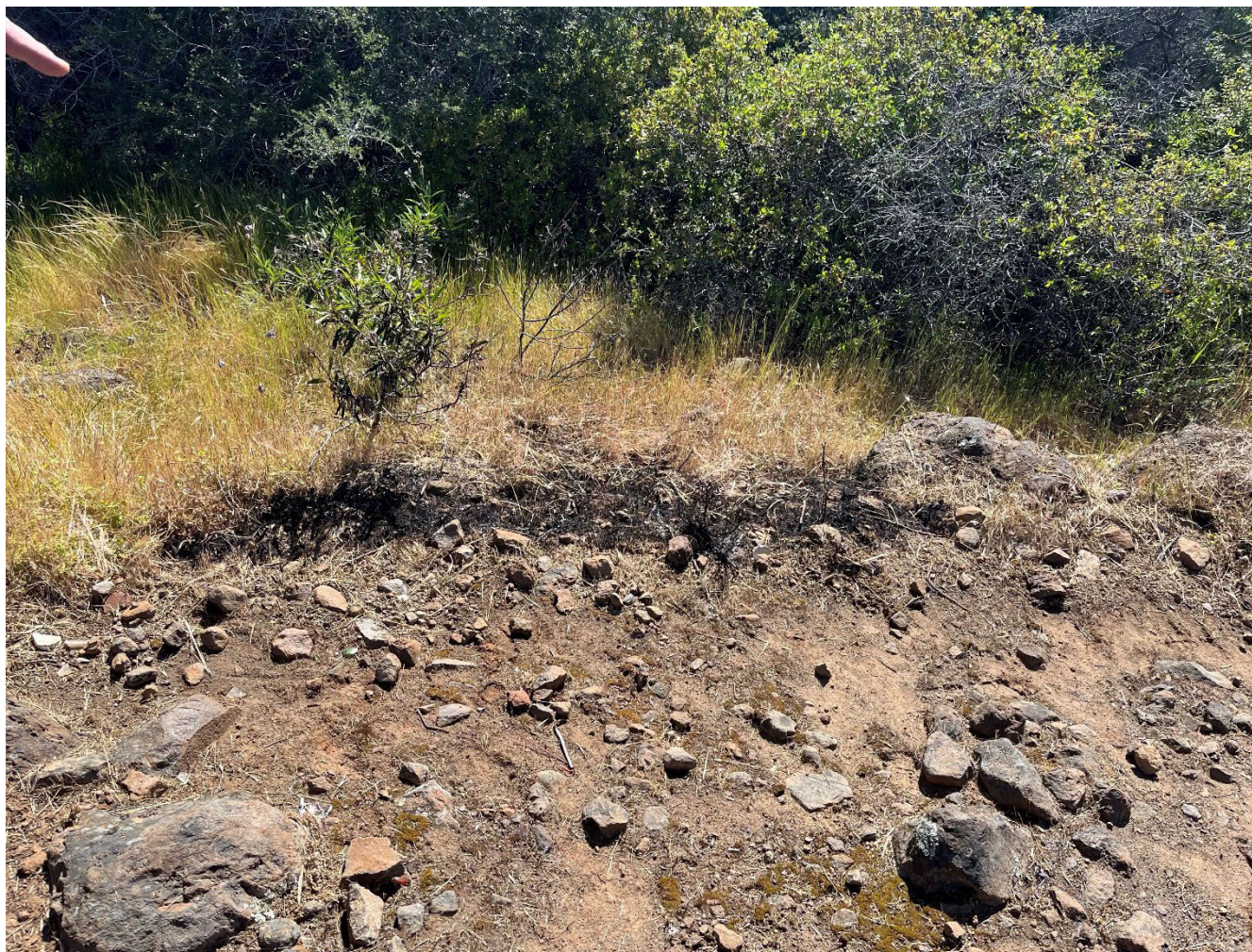
Figure 9 Burn scar at Incident Location #1 - Pole #1. Burn scar was approximately 6.5' x 1' in size. Photo taken by Ignition Investigator on April 22, 2024.
