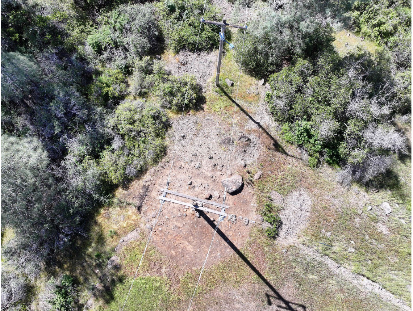
Figure 7 Aerial view of Incident Location #1 - Pole #1 (SAP Pole ID 100331947, with Fuse 26501), showing the defensible space and burn scar just outside of it. Aerial drone photo taken by Ignition Investigator on April 22, 2024.
