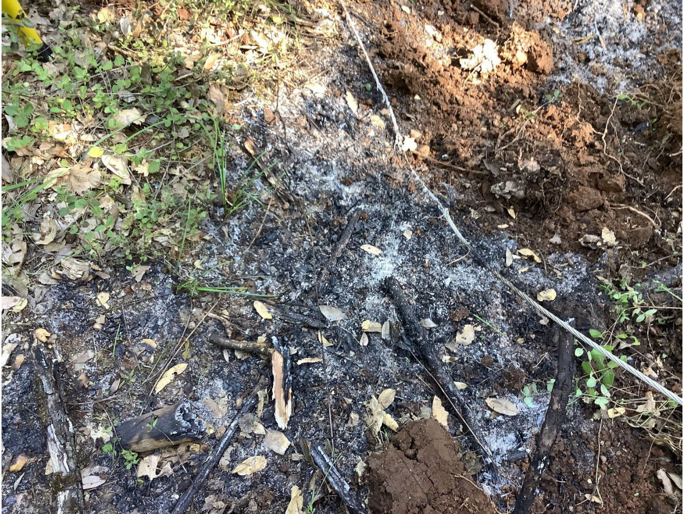
Figure 3 A small section of conductor (footage unknown) still suspended from Pole #2 (behind, to the right in photo). The conductor had melted where it came into contact with the ground. Photo taken by troubleshooter on April 20, 2024.
