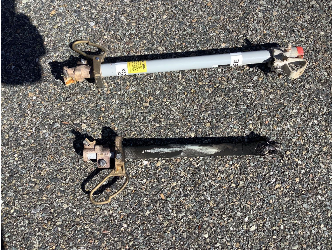
Figure 10 E-fuses that were retrieved from Pole #1 - Incident Location #1. The partially burnt fuse and the sister fuse were sent to ATS for further analysis. Photo taken by troubleshooter on April 20, 2024.
