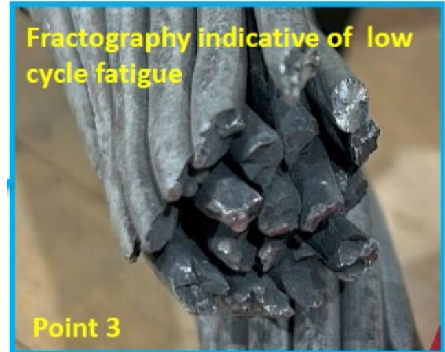
Figure 10 ATS photo of the section of jumper that remained in the dead-end clamp/shoe.
