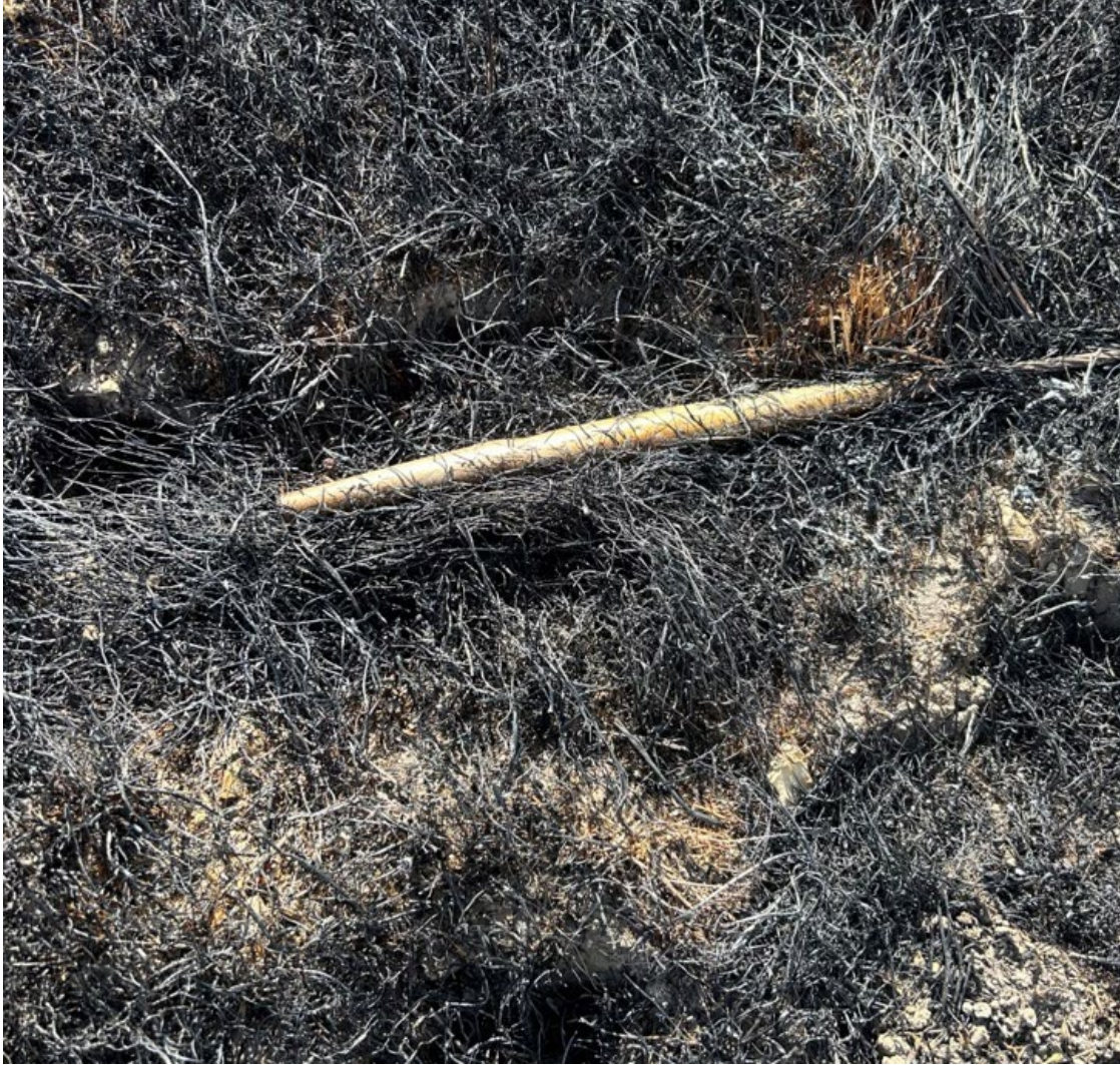
Figure 8 – Photo of failed connector/splice taken by troubleshooter 09/16/2024.
