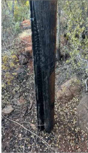
Figure 7 - Secondary service hot-leg connector burned/flushed from overloading on the service which caused arcing and burned the pole and vegetation below.
