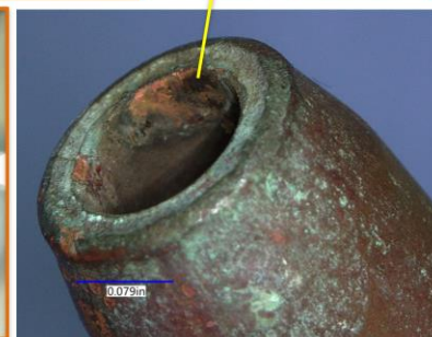
Figure 5 - The failure of the #6 copper conductor occurred at the automatic dead-end connector. The visual inspection of the damaged conductor shows flat fracture consistent with mechanical fatigue. Slide taken from the ATS Summary-Mesa 1101 Conductor Analysis.
