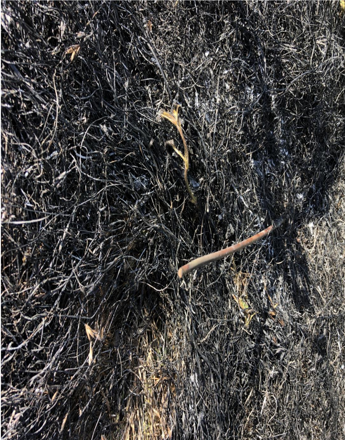
Figure 4 – Source side downed conductor phase end of the Mesa 1101 12kV distribution circuit. Picture taken by the troubleshooter on February 27, 2024.
