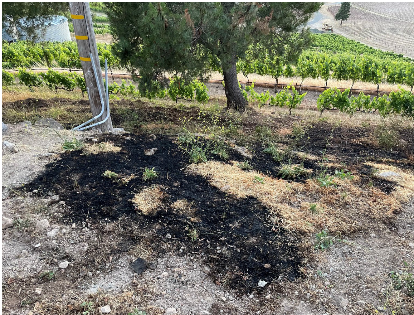
Figure 3 Burn scar at the base of Pole #1. Photo facing south, taken by troubleshooter on June 20, 2024.
