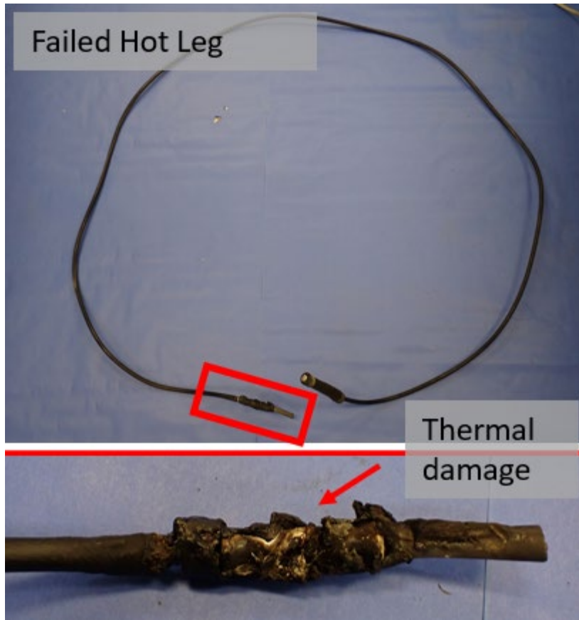
Figure 8 Failed hot leg. Photo taken at ATS by engineer who analyzed the incident.
