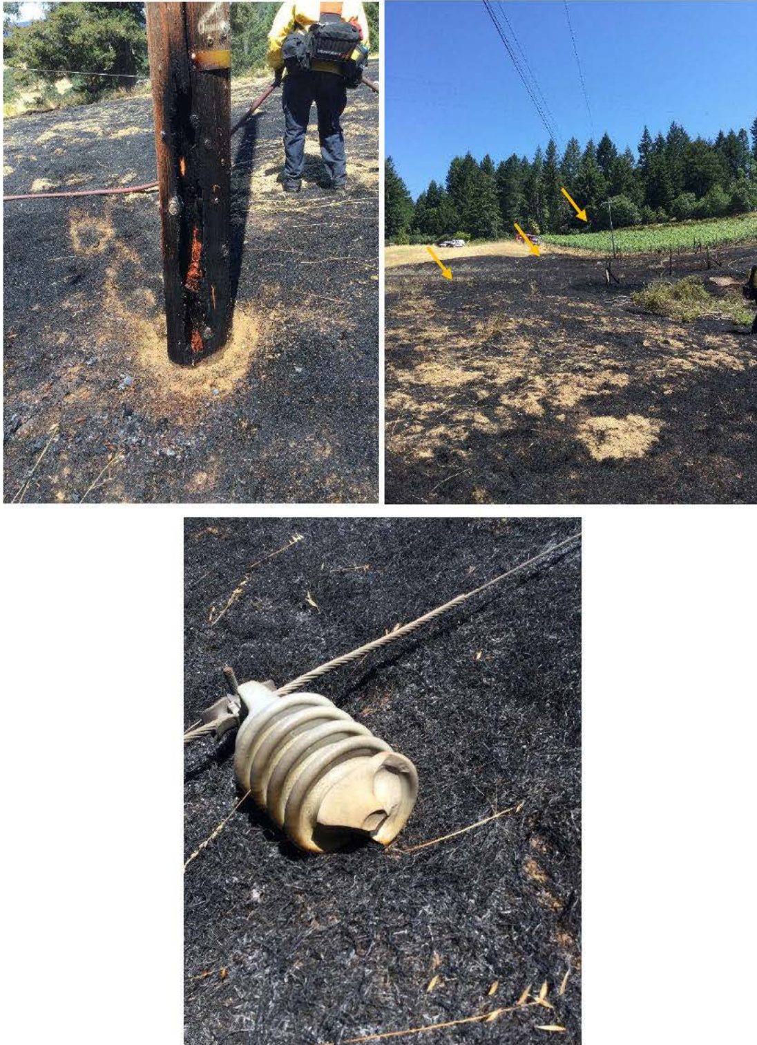
Figure 3 Photographs of damaged Incident Pole (top left), extent of vegetation fire looking towards source side Pole # 2 from the Incident Pole (top, right) and the failed insulator (bottom). Arrows in top right photograph indicate downed wire. Source: Google Maps, image undated.
